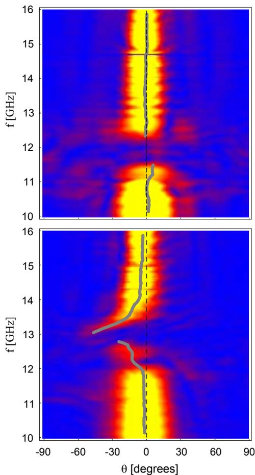
Fig. 5. Angular maps versus frequency of the power emerging from (a) an SRR sample, five unit cells in thickness, with no index gradient and (b) an SRR sample, eight unit cells in thickness, with linear gradient in the direction transverse to the incoming beam.
