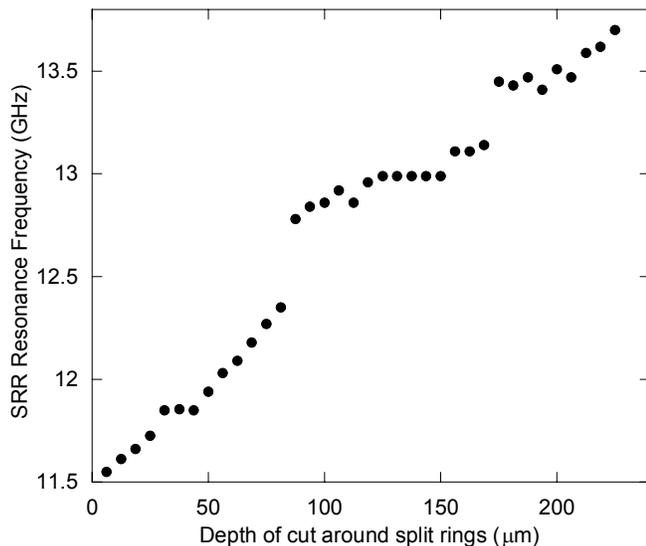
Fig. 4. Resonant frequency versus substrate depth for the machined SRR samples.
