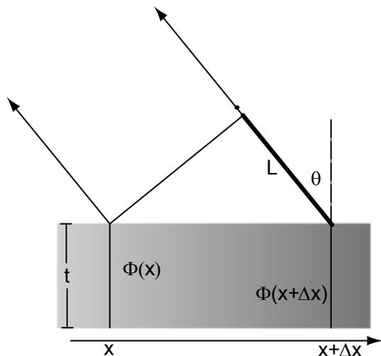
Fig. 2. Diagram showing the deflection of a wave by a structure whose refractive index possesses a gradient that is constant.
