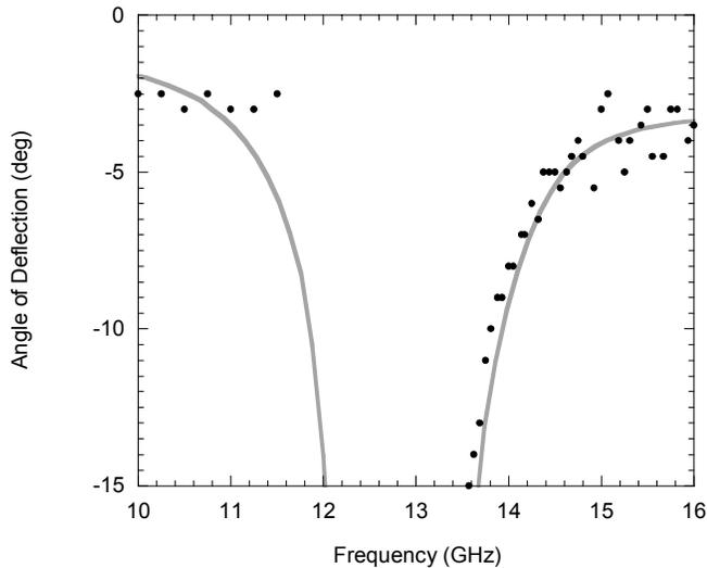
Fig. 6. Measured angle of deflection (black circles) of a gradient index SRR slab, eight unit cells in thickness. The gray curves are taken from those shown in Fig. 3, but have been translated in frequency so that the calculated and the measured band gap regions overlap.
