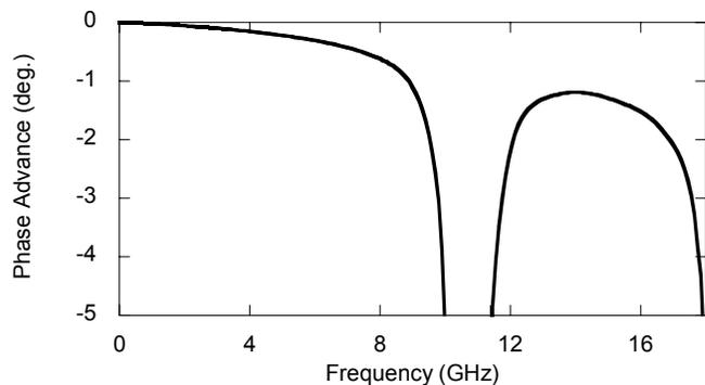
Fig. 3. Frequency versus phase difference per unit cell for the SRR material shown in Fig. 1, in which each successive cell differs by a  $6 \mu\text{m}$  depth of cut.
