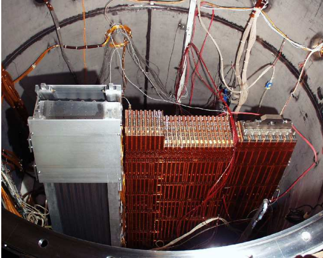
Fig. 2. Top view of the cryostat, showing (from left to right) the EMEC module with the presampler, the three HEC1 modules and the two HEC2 modules of reduced longitudinal size.
