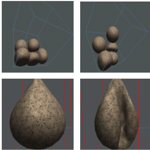
Figure 1: Real time animations created using presented model. Each ball object contains: 320 faces (162 vertices). Both examples run realtime on 800Mhz Duron processor machine (approximately 40-50fps, depending on collision detection configuration).
