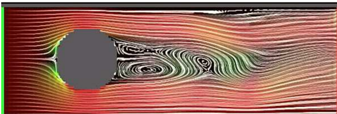
Rysunek 15: A Vortex-Karman Street. Calculation made for Re = 400 and grid size 119 \times 40 .
