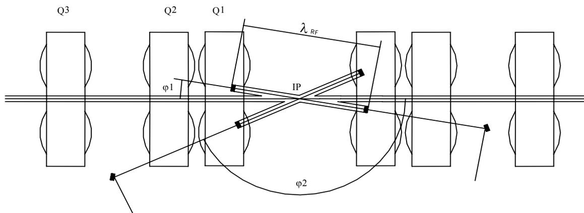
Fig.13. Arrangement of the equipment on IP drift. Collision angles  $\varphi_1 = 10^\circ$  and  $\varphi_2 = 150^\circ$ .
