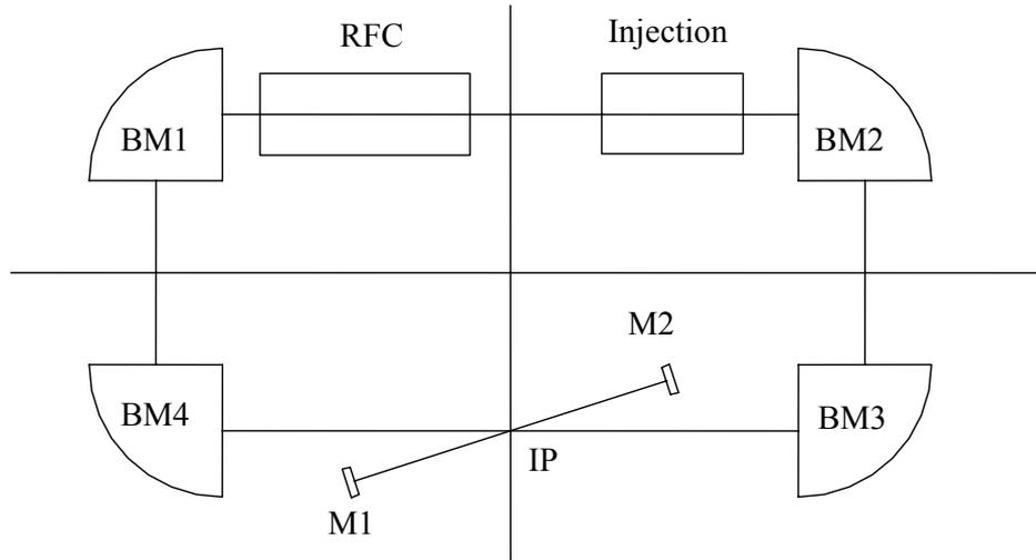
Fig.1. Compact LESR scheme. BM1-BM4 are the bending magnets, IP is the interaction point, M1-M2 are the optical mirrors, RFC is the RF-cavity.
