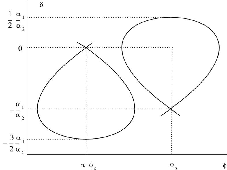
Fig.2. Separatrices of the normal and anomalous beams in case  $|\alpha_2| > \alpha_{2C}$ .
