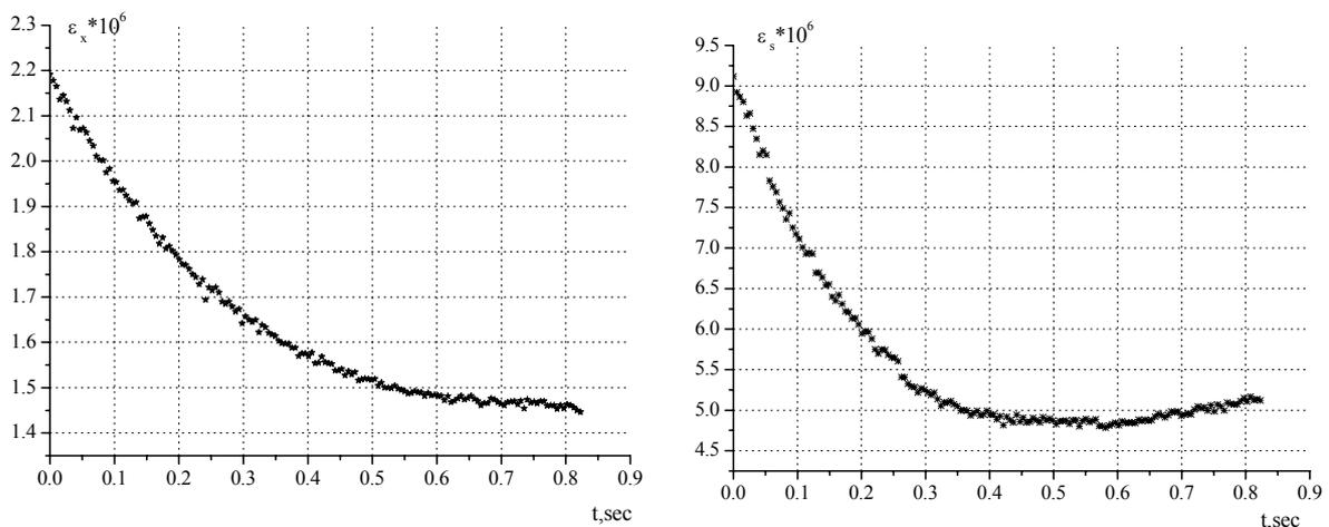
Fig.4. Behavior of horizontal and longitudinal beam emittances involving both radiation damping and IBS.
