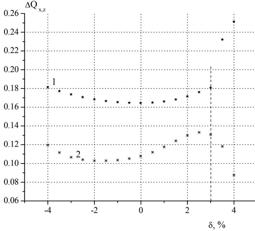
Fig.11. Fractional part of betatron frequencies vs. momentum deviation. Betatron amplitudes at IP are  $x_b = 1$  mm,  $z_b = 0.5$  mm. Vertical dash line bounds range of stable beam motion for  $\delta > 0$ .
