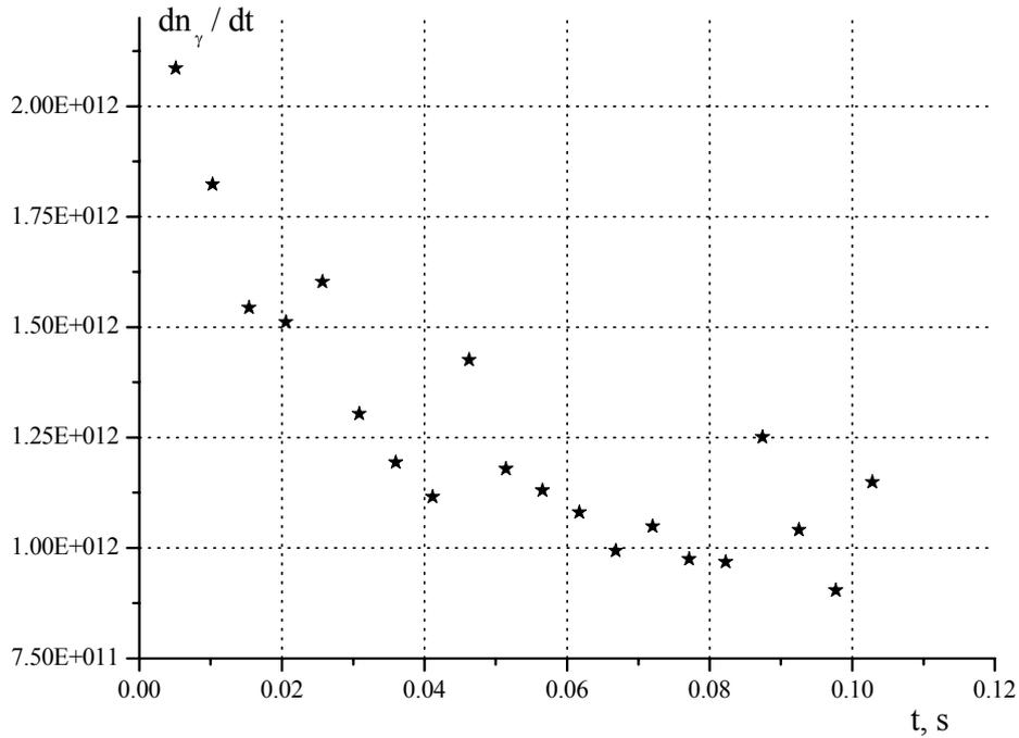
Fig.14. Compton beam intensity during injection interval. Electron beam energy  $E_0 = 43$  MeV, bunch stored current  $I_{\text{stor}} = 10$  mA, bunch number  $n_b = 18$ , stacked laser flash energy  $w_{\text{las}} = 1$  mJ, collision angle  $\varphi = 10^\circ$ , laser beam size  $\sigma_{\text{las}} = 40 \mu$ .
