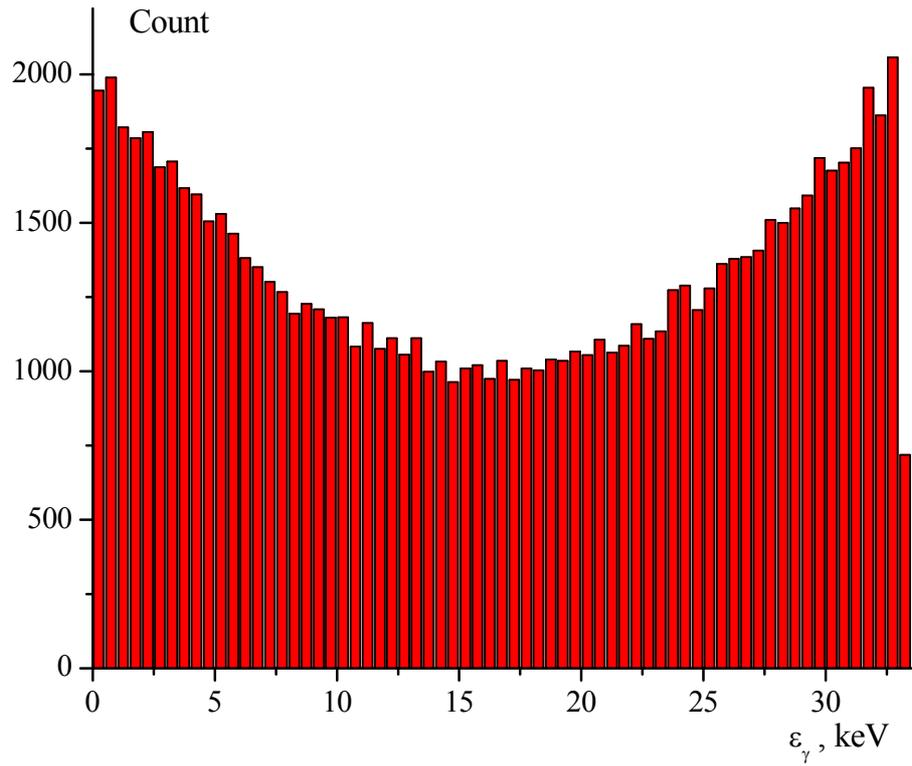
Fig.15. Spectrum of scattered photons within  $4\pi$ -solid angle. Electron beam energy  $E_0 = 43$  MeV, collision angle  $\varphi = 10^\circ$ .
