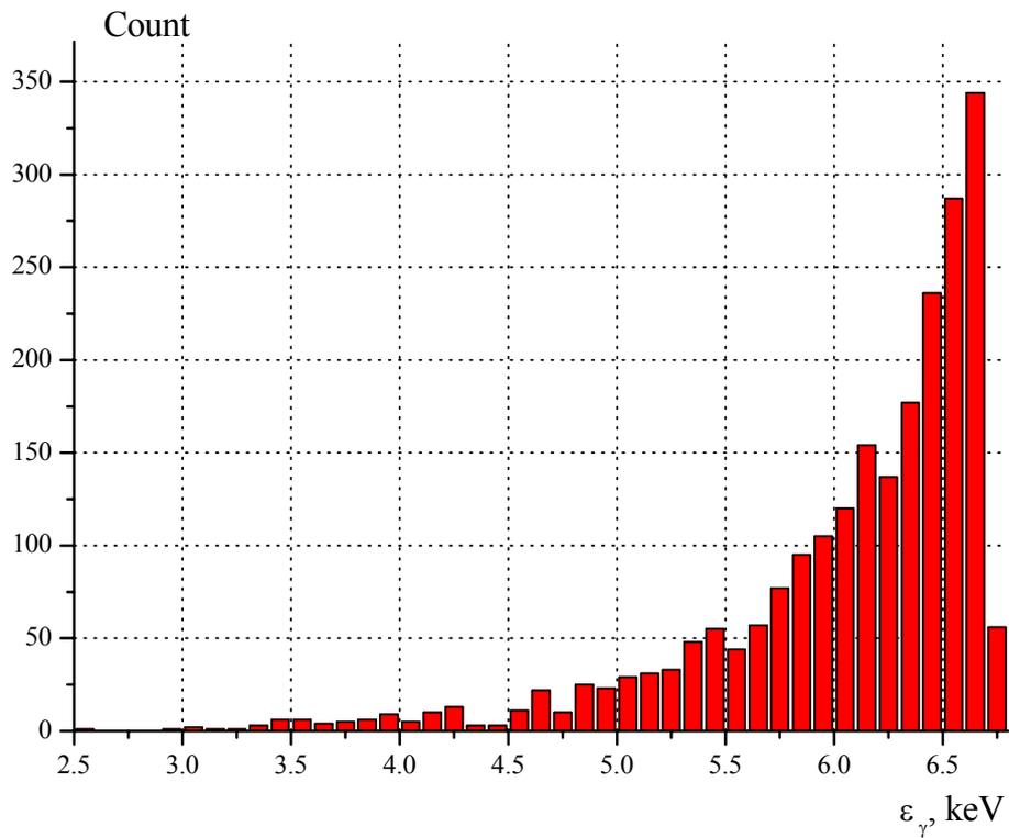
Fig.16. Scattered photons spectrum within collimation angle  $\alpha_{\text{col}} = 1$  mrad. Electron beam energy  $E_0 = 75$  MeV, collision angle  $\varphi = 150^\circ$ .
