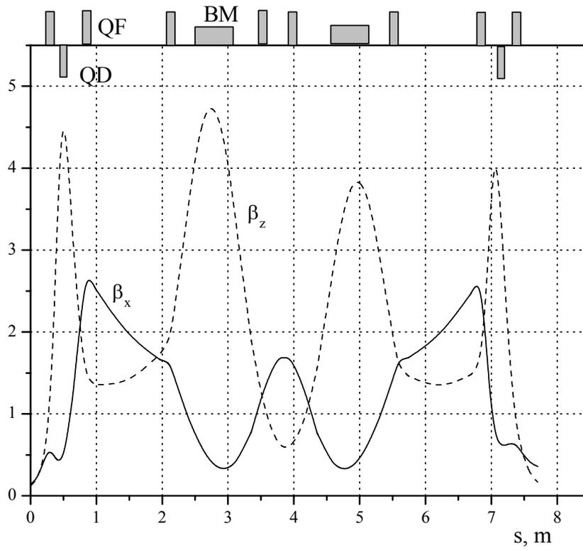
Fig.6. Horizontal  $\beta_x$  and vertical  $\beta_z$  amplitude functions at half ring lattice.
