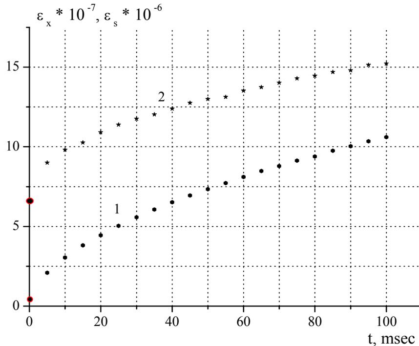
Fig.12. Horizontal (1) and longitudinal (2) emittances during injection interval. Electron beam energy  $E_0 = 43 \text{ MeV}$ , coupling coefficient  $\kappa = 0.05$ , bunch current  $I_{\text{stor}} = 10 \text{ mA}$ .
