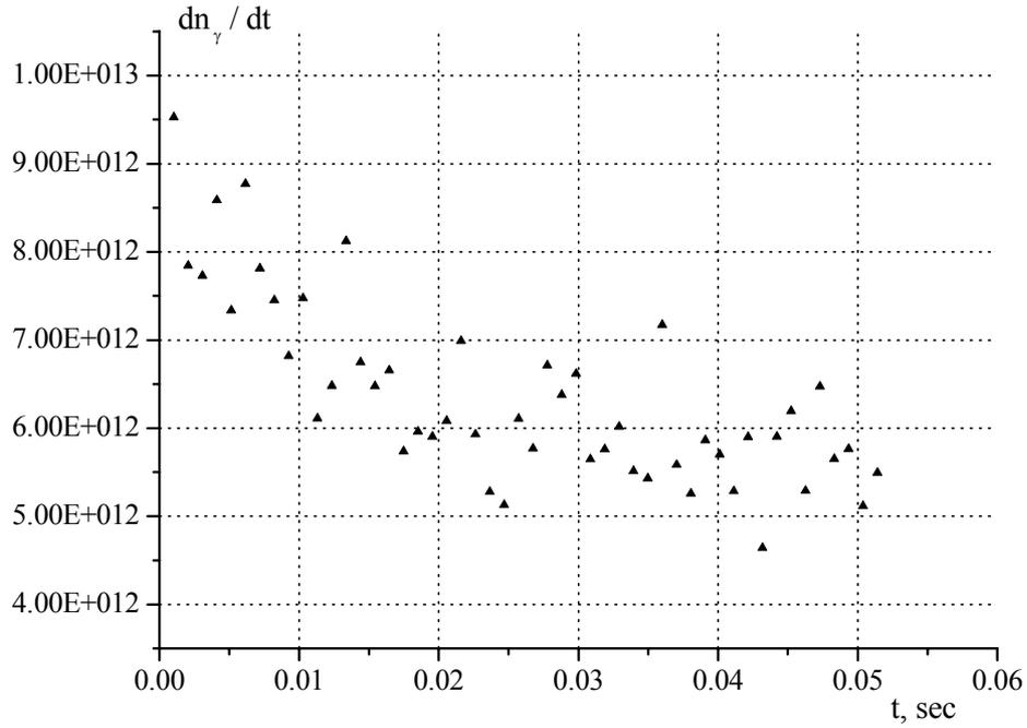
Fig.17. Compton beam intensity. Electron beam energy  $E_0 = 225$  MeV, stored bunch current  $I_{\text{stor}} = 10$  mA, number of electron bunches  $n_b = 18$ , stacked laser flash energy  $w_{\text{las}} = 1$  mJ, collision angle  $\varphi = 10^\circ$ .
