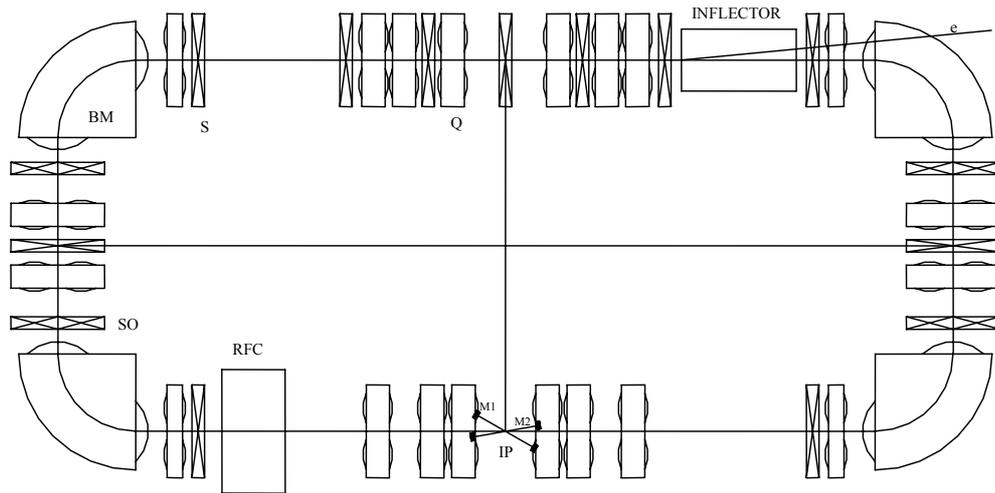
Fig.5. NESTOR layout. IP is the interaction point, BM are the bending magnets, Q, S, SO are the quadrupole, sextupole and combined sextupole and octupole lenses, correspondingly, RFC is the RF-cavity, Inflector is the injection kicker magnet, M1-M2 are the mirrors of the optical cavity.
