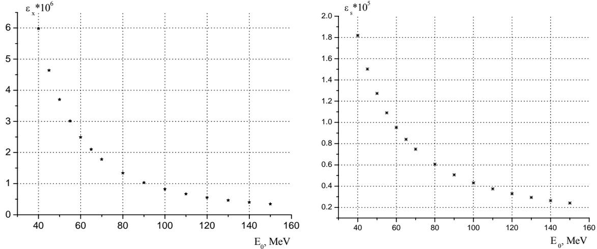
Fig.3. Dependencies of horizontal and longitudinal emittances on electron beam energy at stored bunch current  $I_{stor} = 10$  mA.
