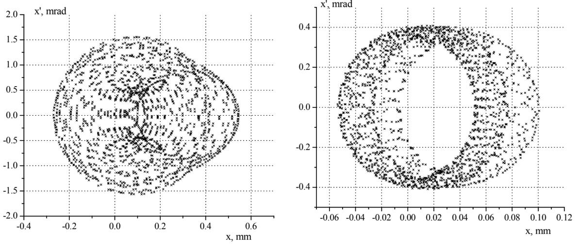
Fig.8. Horizontal phase trajectories of particle with large momentum deviation at IP azimuth in operation modes with large and low momentum compaction factor ( $\alpha_1 = 0.078$  and  $\alpha_1 = 0.019$ , correspondingly). Initial particle coordinates are
