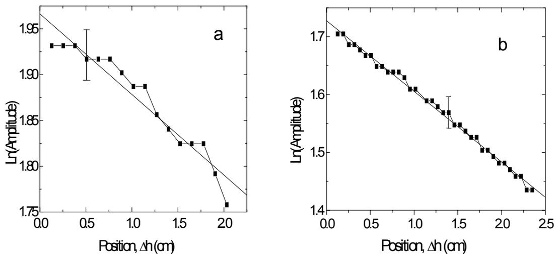
Fig.7. Amplitude of the transmitted ultrasonic signal as a function of sample length (position of the upper buffer rod). a,  $T=120\text{ }^{\circ}\text{C}$ ; b,  $T=170\text{ }^{\circ}\text{C}$ . See text for details.
