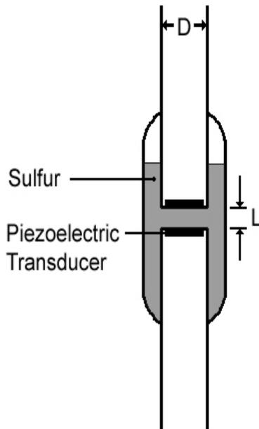
Fig. 1. Schematic diagram of the quartz cell for measurements of sound velocity.
