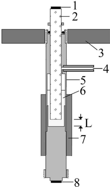
Fig. 2. The cell used for measurements of sound absorption.
