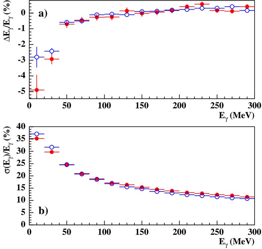
Fig. 16. Energy response and resolution determined using  $\phi \rightarrow \pi^+\pi^-\pi^0$  events with photons incident on the calorimeter barrel: a) relative linearity of energy response,  $\Delta E_\gamma/E_\gamma$ , as a function of  $E_\gamma$ ; b) relative energy resolution,  $\sigma(E_\gamma)/E_\gamma$ , as a function of  $E_\gamma$ . Solid (open) circles are for data (MC).
