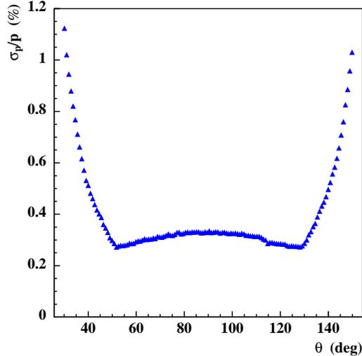
Fig. 4. Momentum resolution  $\sigma_p/p$  as a function of polar angle  $\theta$ , for Bhabha events.
