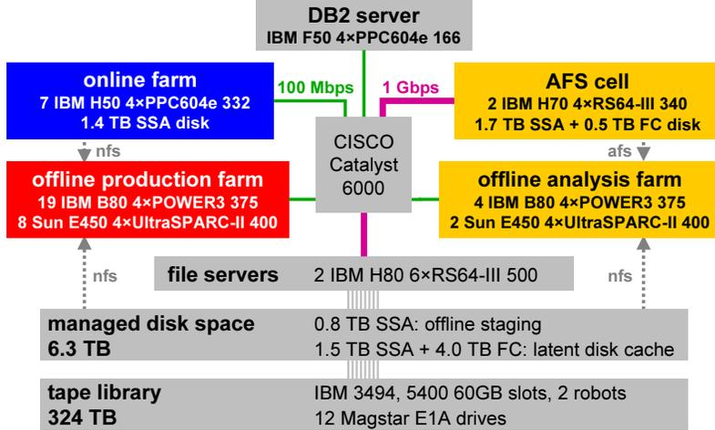
Fig. 1. KLOE computing hardware configuration during 2001–2002.
