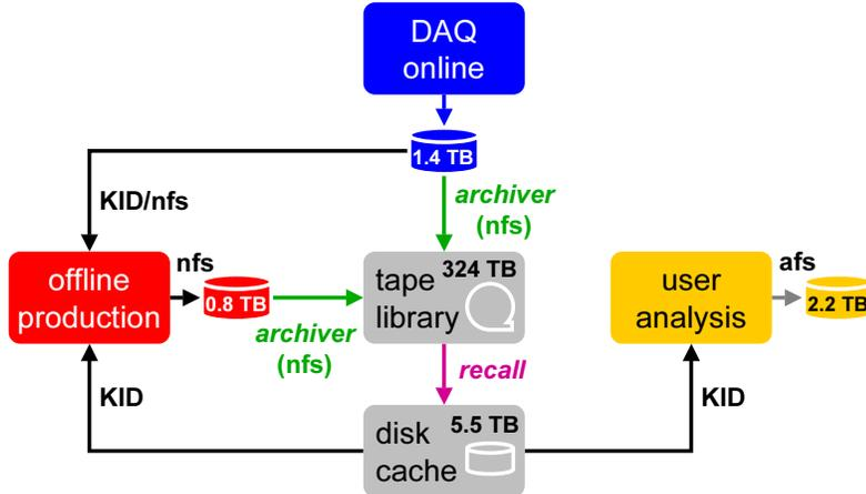
Fig. 3. Schematic layout of KLOE data handling.
