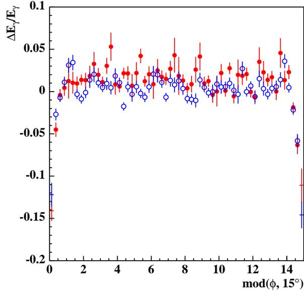
Fig. 17. Energy response as a function of the azimuthal distance from the boundaries between modules of the barrel calorimeter. Solid (open) circles are for data (MC).
