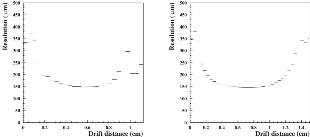
Fig. 8. Spatial resolution as a function of the impact parameter for small (left) and large (right) cells.
