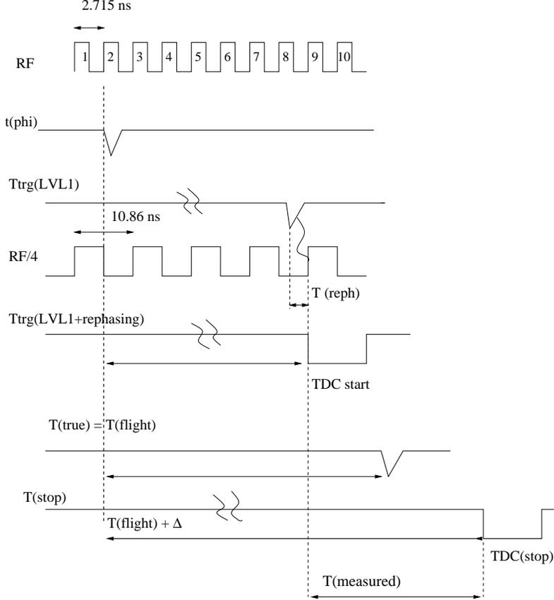
Fig. 10. Timing scheme for bunch-crossing signal, calorimeter signals, and level-1 trigger formation.
