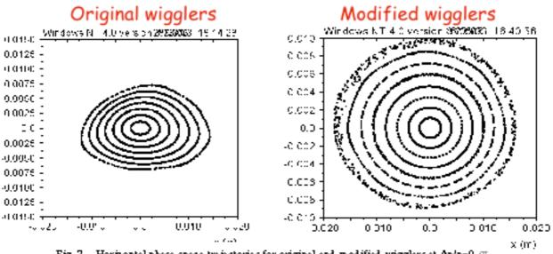
Fig. 7 – Horizontal phase space trajectories for original and modified wigglers at  $\Delta p/p=0$ ,  $\pi$  .
