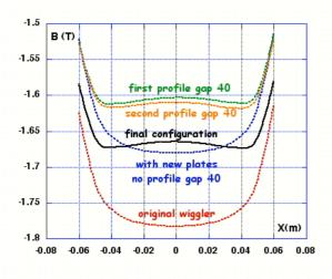
Fig. 5 - horizontal field distribution at pole center for different configurations. The solid line is the final one.
