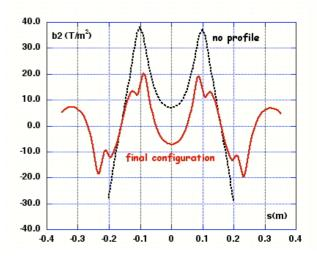
Fig. 6 - Sextupole component on the beam axis for the original (dashed) and modified (solid) wiggler pole profile.
