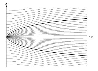
FIG. 5: Flux lines of the vector field  $\vec{j}(\vec{r})$  in the x-z plane for the three-dimensional problem. The separatrix between flux lines terminating at the target charge and those terminating elsewhere at the wall is represented as a bold line. In the two-dimensional case one obtains a qualitatively similar flow field.
