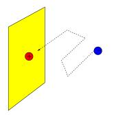
FIG. 3: Simplified model for electrostatically supported coating: A negatively charged pointlike particle is attracted by a positive charge located at the planar surface of an infinitely large spherical particle.
