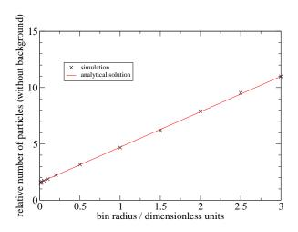
FIG. 7: Influx of particles onto the wall within a circular shaped region around the fixed charge. The straight line represents the analytical solution:  $\frac{\pi}{2} + \pi R$ . In both cases, the constant background is subtracted.
