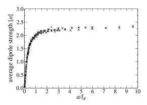
FIG. 10: Agglomeration of two spherical particles: Average dipole strength in units of particle radii a as function of the particle radius in units of the Bjerrum length  $l_B$ . For particle radii bigger than the Bjerrum length, the position of charges during agglomeration is randomized due to Brownian rotation.
