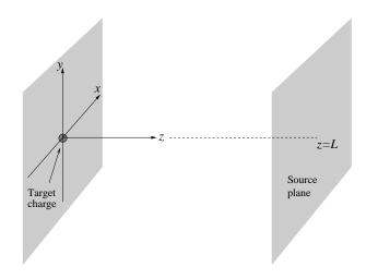
FIG. 4: A thermally diffusing particle inserted randomly at finite distance z=L is attracted by the target charge at the origin. Once the particle touches the target plane z=0, which represents the large particle to be coated, it sticks to its surface due to van-der-Waals forces. The single-particle problem can be recast as a quasi-stationary flow of a large number of particles inserted continously along the source plane which are removed whenever they touch the target plane.
