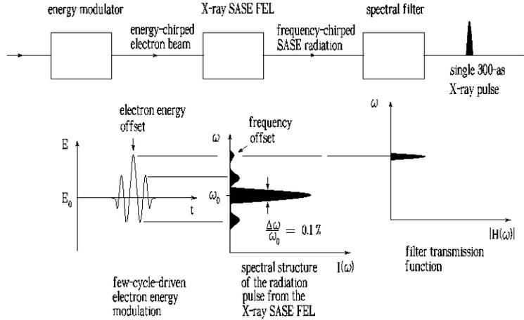
Fig. 2. Sketch of single attosecond X-ray pulse synthesis through frequency chirping and spectral filtering
