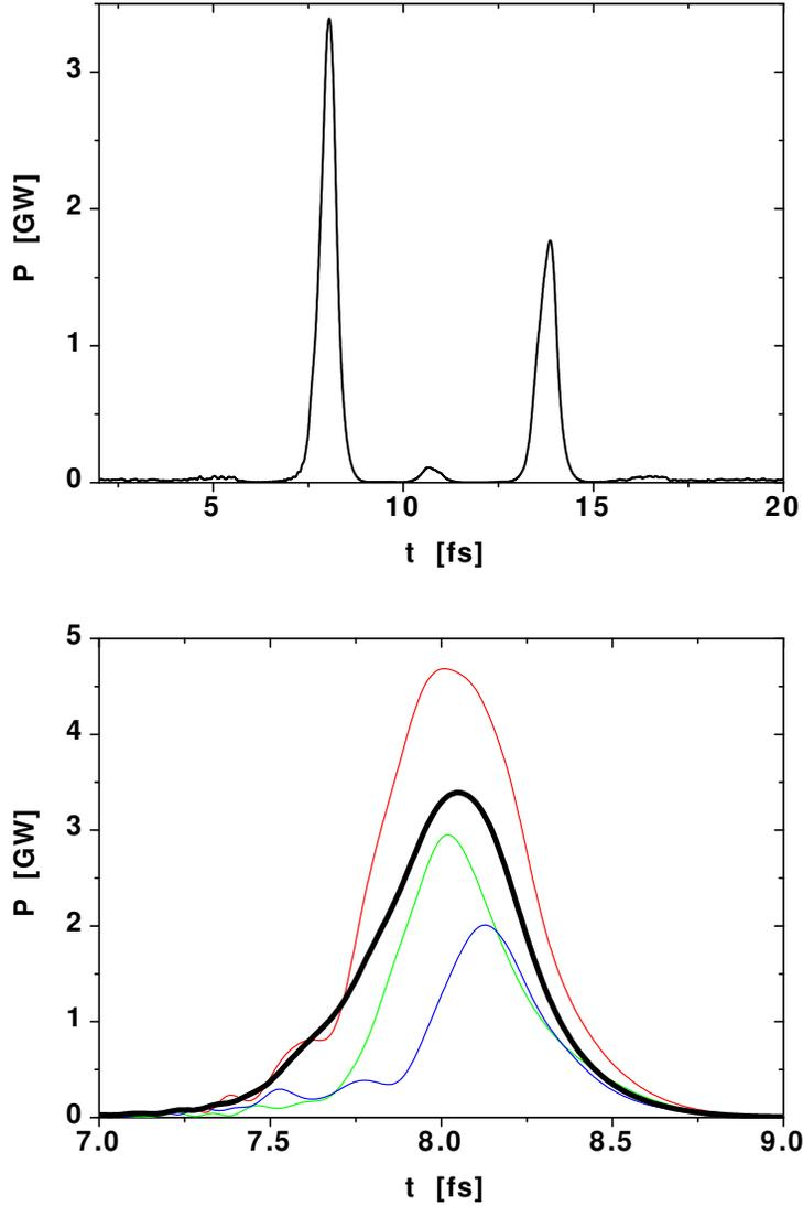
Fig. 12. Temporal structure of the radiation pulse behind monochromator tuned to selection of two pulse sequence (mark  $M_2$  in Fig. 10). Pulse separation is two laser oscillation periods. Upper plot shows average over many pulses, and lower plot shows details of single pulses. Bold curve is average over many pulses
