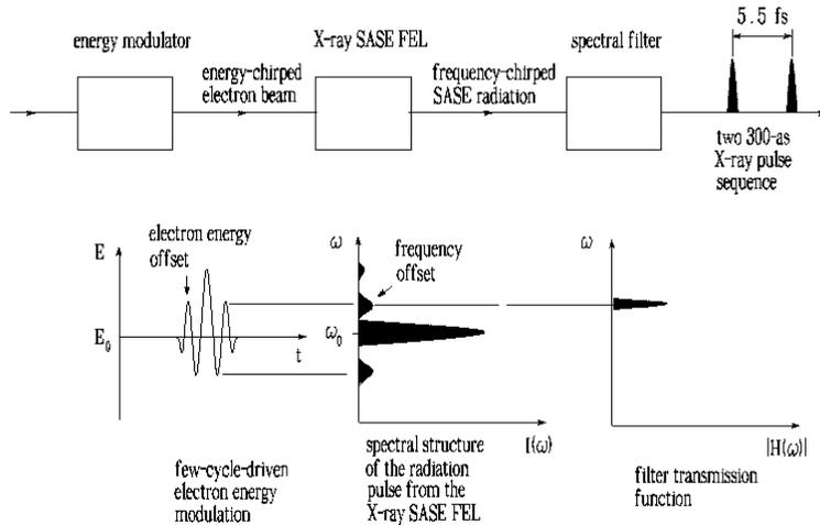
Fig. 3. Sketch of two attosecond X-ray pulse sequence synthesis through frequency chirping and spectral filtering. Pulse separation is  $2T_0$ , where  $T_0$  is the Ti:sapphire laser oscillation period
