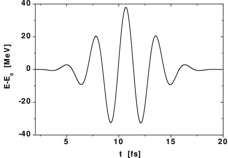
Fig. 5. Energy modulation of the electron beam at the exit of the modulator undulator. The laser parameters are  $\lambda = 800$  nm,  $W_{\text{peak}} = 800$  GW, and FWHM pulse duration of  $\tau_p = 5$  fs
