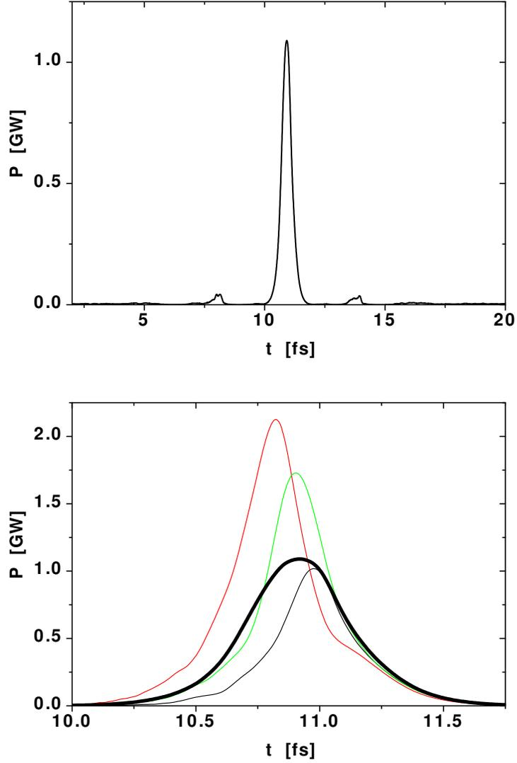
Fig. 11. Temporal structure of the radiation pulse behind monochromator tuned to single spike selection (mark  $M_1$  in Fig. 10). Upper plot shows average over many pulses, and lower plot shows details of single pulses. Bold curve is average over many pulses
