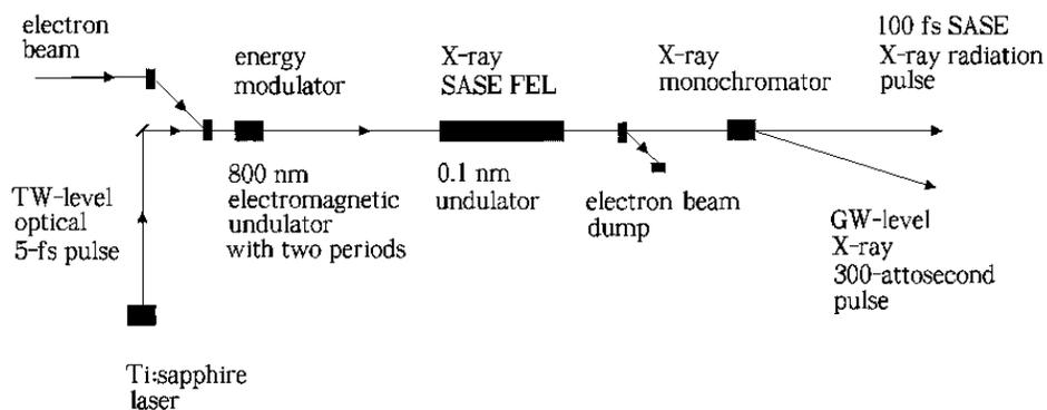
Fig. 1. Schematic diagram of attosecond X-ray source
