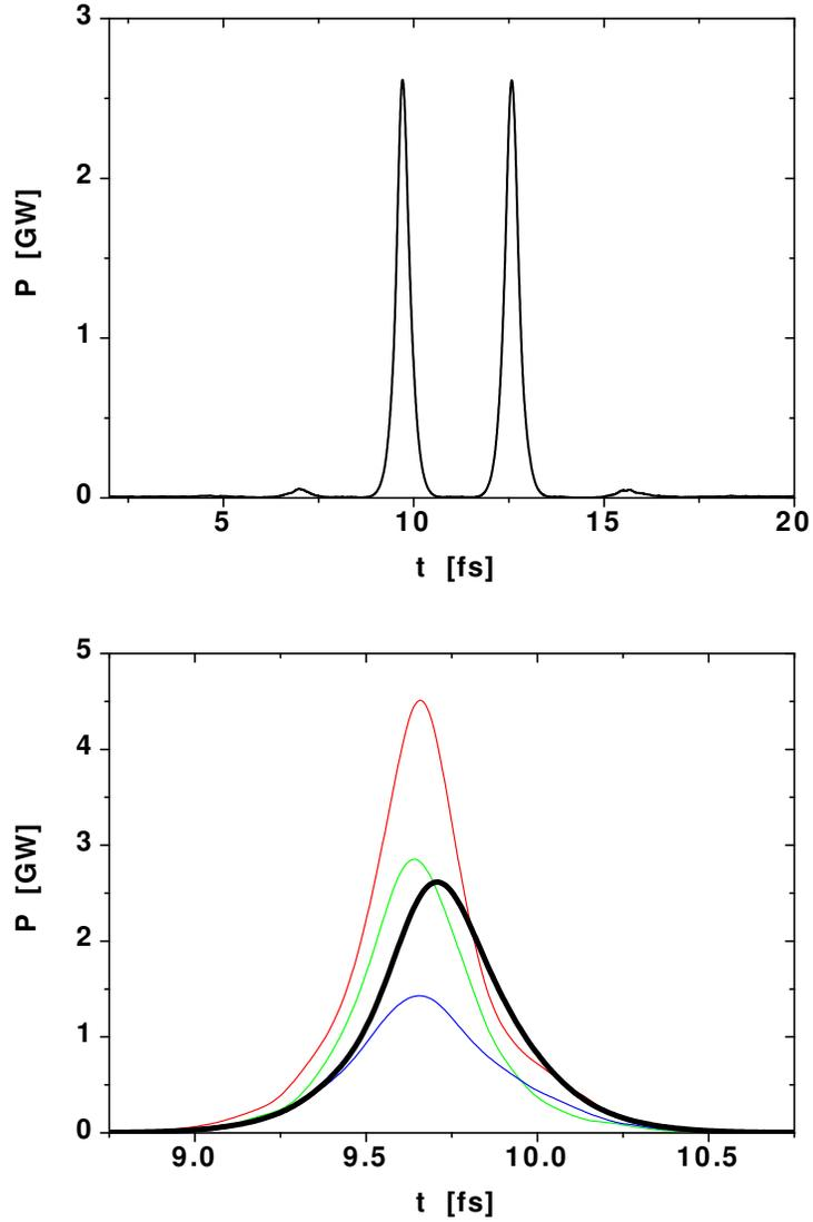
Fig. 13. Temporal structure of the radiation pulse behind monochromator tuned to selection of two pulse sequence (mark  $M_3$  in Fig. 10). Pulse separation is one laser oscillation period Upper plot shows average over many pulses, and lower plot shows details of single pulses. Bold curve is average over many pulses
