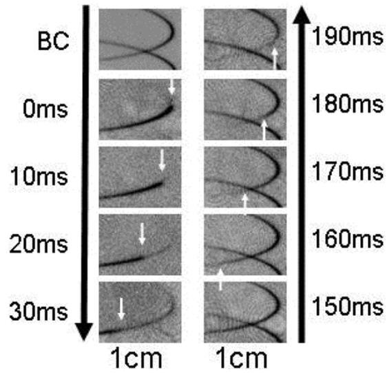
Figure 5: Absorption images near the right curve of the stadium. “BC” = “Before Cut”, taken 100 ms after SW operation. The images taken at  $t' = t - 105$  ms (0 ms to 30 ms after cut) show the edge of the cloud propagating “down-left” (clockwise). The images from  $t' = 150$  ms to 190 ms show the edge propagating “right-up” (counterclockwise). This indicates bidirectional propagation around the entire ring. White arrows were added to clarify the edge of the atom cloud.
