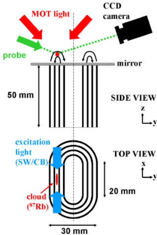
Figure 1 (Color Online): Top: Photograph of the stadium-assembly (without mirror). Kapton<sup>®</sup> wires are wrapped around each foil and attached to the mu-metal with Torr Seal glue<sup>®</sup>. Bottom: top view and side view of the experimental setup. Same laser beam is used for standing wave (SW) operation ( $\delta = +7\Gamma$ ) and as a cutting beam (CB, on-resonance).
