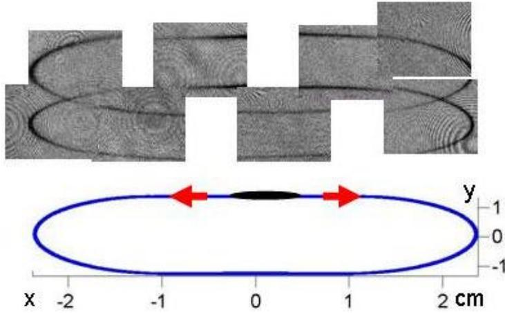
Figure 4: Top: Sequence of absorption images of trapped atoms along the circumference of the stadium after 200 ms of free evolution. Observation angle ( $\sim 18^\circ$ ), magnification (1:1) and grayscale of each image may vary slightly. Mirror image is also visible. Bottom: Calculated isopotential surface of  $|B|=2$  Gauss, the observation angle is set to be  $18^\circ$ . The initial distribution and propagation directions of atom sample are also indicated.
