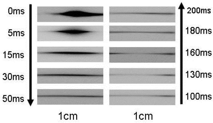
Figure 3: a) Evolution of the atom cloud in the straight part of the stadium after loading at  $t = 0$  ms. Two groups of atoms which make 30% of total atom number come back at around  $t=160$  ms, due to back-scattering from the curved parts.
