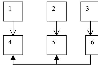
**FIGURE 2.** Electronics setup. 1,2-Receivers; 3-Atomic clock; 4,5-Counters; 6-Scaler.
