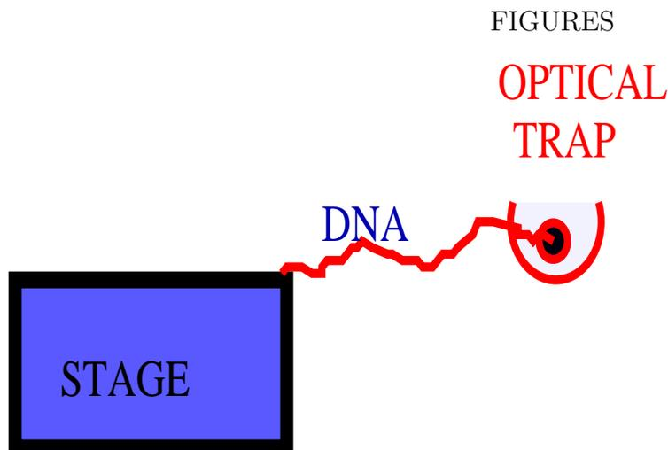
FIG. 1. Schematic Experimental Setup for a Typical Force Extension Measurement.
