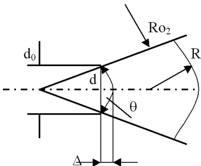
Fig. 1. Angle of the beam divergence.
