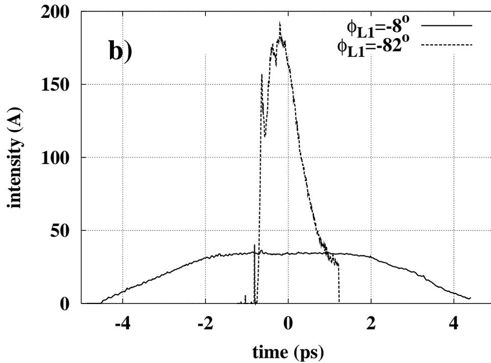
FIG. 6: Comparison of the bunch time-profile for L1 on crest ( $\phi_{L1} = 0^\circ$ ), and  $-82^\circ$  off-crest. Plot **a)** was generated by tracking simulation; plot **b)** is a direct measurement using the zero-phasing method. The time  $> 0$  corresponds to the bunch tail
