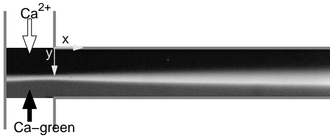
FIG. 3: Fluorescent microscopy image of the binding of \text{Ca}^{2+} ions with Calcium-green marker in a T-channel. The channel width is 200 \mu\text{m} , the depth is 10 \mu\text{m} . Here, the velocity in the main channel is U = 0.083 \text{ cm/s} .
