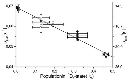
FIG. 6: Decay rates  $\alpha_{p=0}$  as a function of the excitation  $\pi_3$  allowing the determination of  $\tau_2$  in the limit of  $\pi_3 \rightarrow 0$ .
