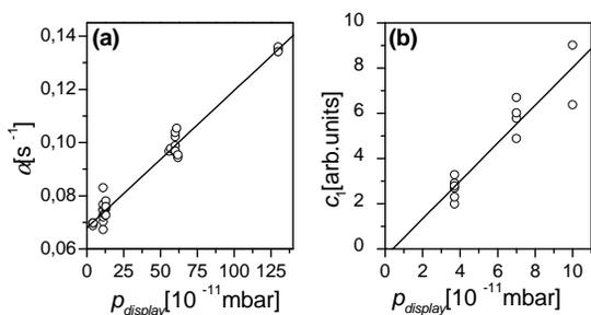
FIG. 4: (a) Decay rates  $\alpha$  obtained for  $\pi_3 < 0.1$  after extrapolation to  $\pi_3 = 0$  as a function of the nominal background pressure  $p_{\text{display}}$ . (b) Coefficients  $c_1$  proportional to the number of ionizing background collisions as a function of  $p_{\text{display}}$  allowing the determination of the vacuum gauge offset.
