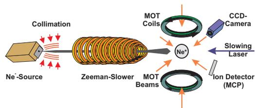
FIG. 3: Experimental setup.
