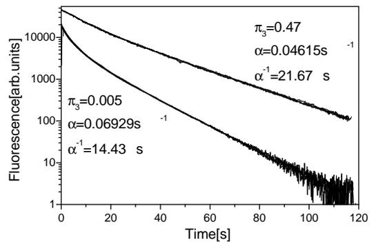
FIG. 1: Decay of the fluorescence for a  $^{20}\text{Ne}$  ensemble in a MOT for the given excitations to the  $^3D_3$  state of  $\pi_3 = 0.005$  ( $\Delta/\Gamma = -5.3$ ,  $I/I_0 = 1.75$ ,  $p = 3.4 \times 10^{-11} \text{ mbar}$ ) and  $\pi_3 = 0.47$  ( $\Delta/\Gamma = -0.16$ ,  $I/I_0 = 24$ ,  $p = 4.7 \times 10^{-11} \text{ mbar}$ ). Both sets of data consist of five curves each, demonstrating the high reproducibility of our decay measurements.
