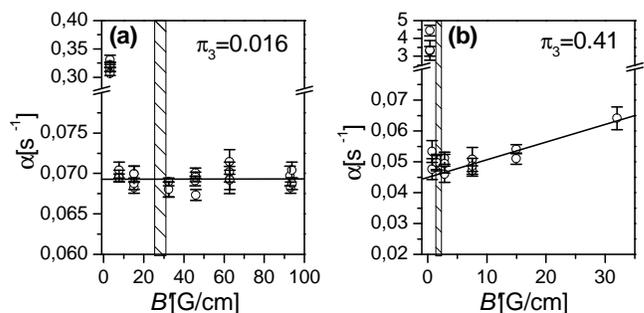
FIG. 5: Systematic investigation of MOT losses. Decay rates are plotted as a function of the magnetic field gradient for two different excitations (a)  $\pi_3 = 0.016$  and (b)  $\pi_3 = 0.42$ . Shaded areas indicate the gradients of typical operating conditions.
