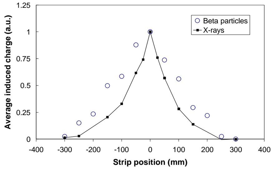
Fig. 6. Induced charge profile for the detection of collimated  $\beta$  particles and X-rays.
