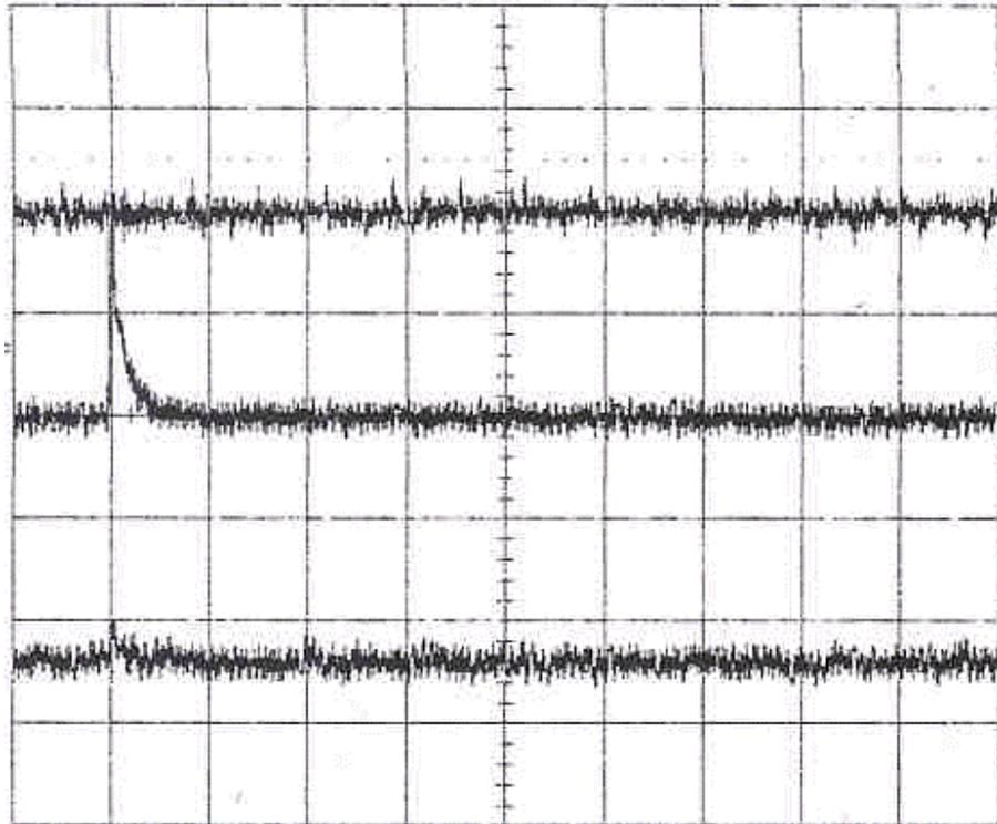
Fig. 5. Signals from three adjusted strips in the case of detection of the cosmic event. Horizontal scale 0.5ms/div; vertical scale 0.5V/div.
