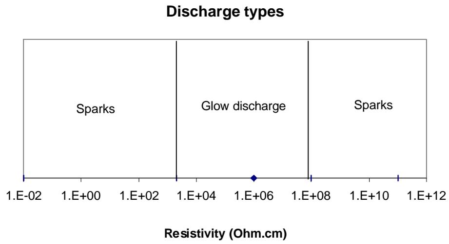
Fig. 4. Types of discharges in RPCs with various electrode resistivities.
