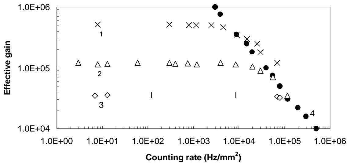
Fig. 3. Gain vs. rate for RPCs made of various low resistivity materials: 1)  $\rho=3 \times 10^8 \Omega \cdot \text{cm}^2$ ; 2)  $\rho=4 \times 10^7 \Omega \cdot \text{cm}^3$ ; 3)  $\rho \sim 10 \times 4 \Omega \cdot \text{cm}$  (GaAs and Si); 4) gain vs rate for metallic PPAC.
