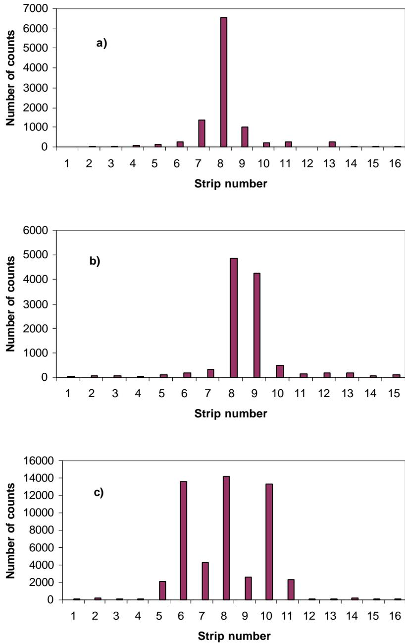
Fig. 7. Number of counts from various strips in the case when X-rays penetrated to the RPC through a 30  $\mu\text{m}$  slit with the beam oriented along the strip #8 (a) and in between the strips #8 and #9 (b). The picture was periodically repeated when the beam was further moved perpendicularly to the strips. c) Number of counts from various strips for X-ray imaging of a 7 lp/mm phantom.
