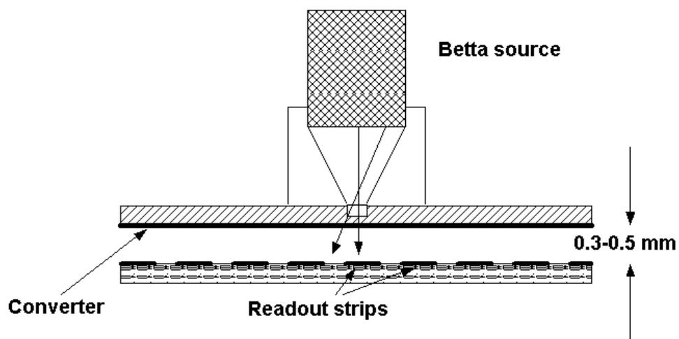
Fig. 2. Schematic drawing of the  $\beta$ -particles collimation setup.
