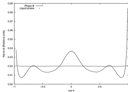
Fig. 5. Orientation distribution  $N(\cos\theta)$  for  $TeF_6(89)$  cluster, with  $q_F = 0.25e$
