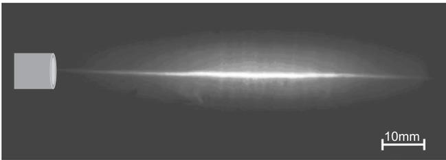
FIG. 2: Picture of the fluorescence in the 2D-MOT with a flux of  $3.5 \cdot 10^{10}$  atoms/s. The vapor pressure in the glass cell is about  $7 \cdot 10^{-7}$  mbar. A beam of approximately 90 mm length and a thickness of 2 mm develops. The cooling region extends to the differential pumping tube which is sketched on the left.
