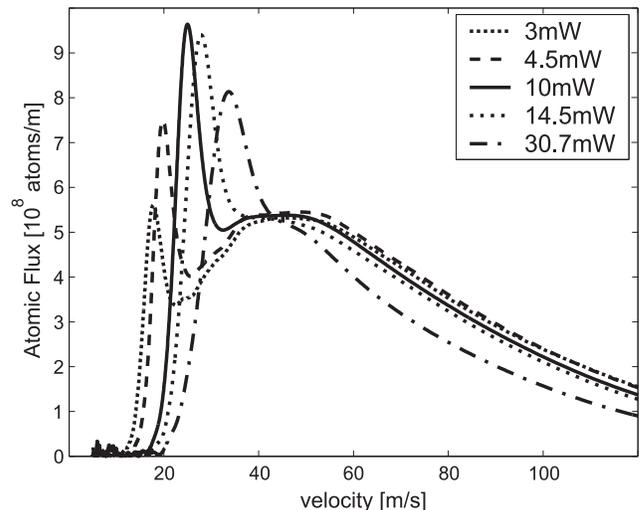
FIG. 10: When a laser beam is shone on the axis copropagating with the atomic beam, the longitudinal velocity distribution changes dramatically. A narrow peak rises up at velocities between 20 m/s and 40 m/s. Its width and position on the  $v_z$ -axis depends on the intensity in the pushing beam. Atoms at very low velocities below 15 m/s are pushed out of the beam or are accelerated. The total flux stays nearly constant.
