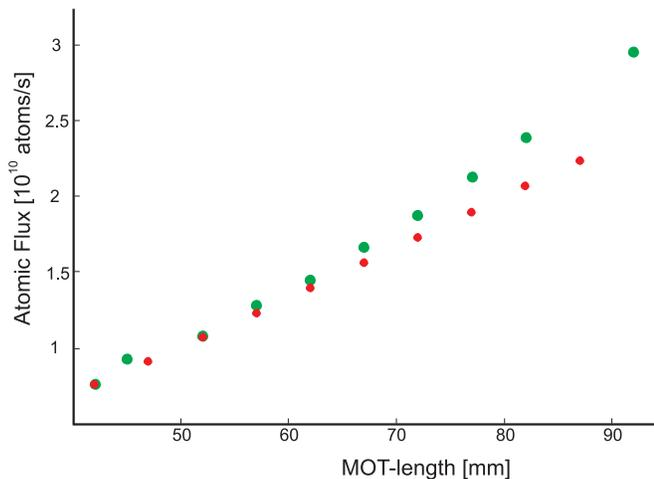
FIG. 7: Dependence of the total flux on the length of the cooling volume. The experimental parameters are the same as in Fig. 6. The dark spots show the theoretical the bright circles the experimental data.
