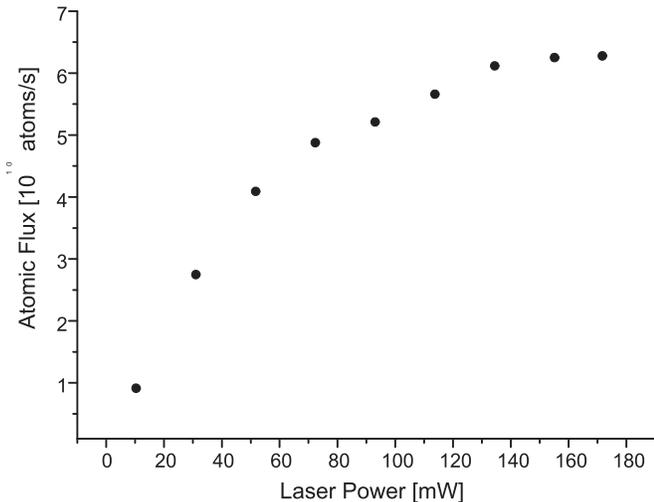
FIG. 5: Dependence of the total atomic flux on the cooling laser power per beam. The total flux in atoms/s is given by the area under the curves in graph 4. It ranges from  $1 \cdot 10^{10}$  to  $6 \cdot 10^{10}$  atoms/s. The total flux depends strongly on laser power and saturates at values of 160 mW per laser beam.
