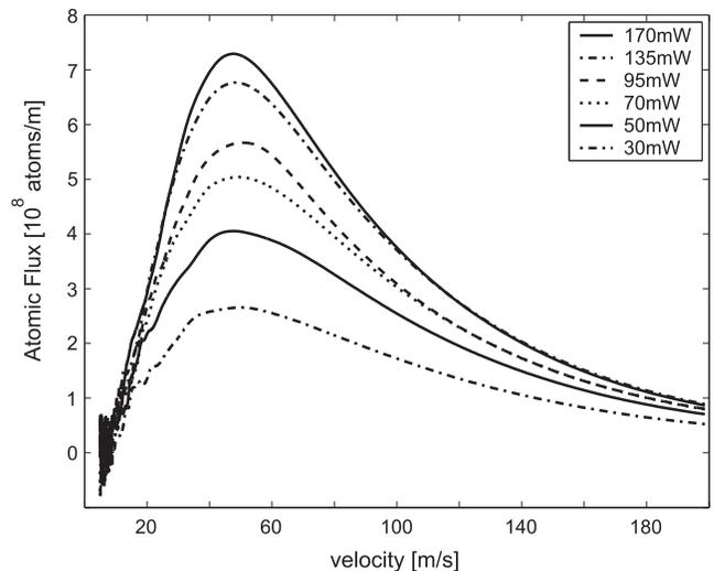
FIG. 4: Distribution of the atomic flux versus the longitudinal velocity. The laser power in the cooling beams was varied from 30 mW to 170 mW. The pressure for this measurement is  $1.6 \cdot 10^{-6}$  mbar, the length is 92 mm. A small shift of the mean velocity to higher values with increasing laser power is visible. The velocity distribution is centered around 50 m/s and has a width of about 75 m/s.
