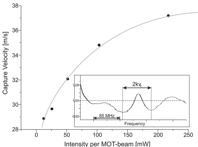
FIG. 3: Transverse capture velocity of the 2D-MOT. The inset shows the normalized Doppler-spectroscopy signal, i.e. the measured signal divided by a fitted Gaussian distribution. The width between the two minima corresponds to twice the capture velocity. The main graph shows the dependence of the capture velocity on the intensity in the cooling laser beams. The line serves merely to guide the eye. The capture velocity saturates at high intensities at a value of 38 m/s.
