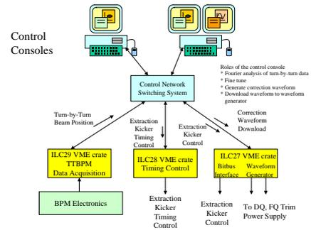
Figure 3. Tune acquisition and correction system.
