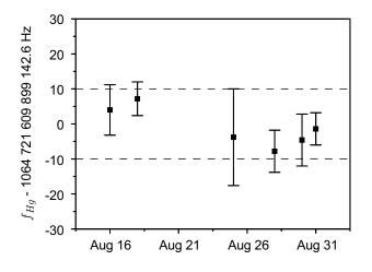
FIG. 3: A chronological record of the average daily frequency of the  $^{199}{\rm Hg^+}$  clock transition measured on six days over a 15 day period representing 21 651 s of total measurement time. The error bars represent statistical fluctuations. The dashed lines represent an estimated systematic uncertainty of  $\pm 10~{\rm Hz}$  in the Hg<sup>+</sup> system in the absence of a full evaluation.
