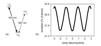
FIG. 2: (a) Simplied diagram of the relevant energy levels in the Ca standard. (b) Optical Bordé-Ramsey fringes with a 960 Hz (FWHM) resolution. The total averaging time to generate this figure was 20 s.
