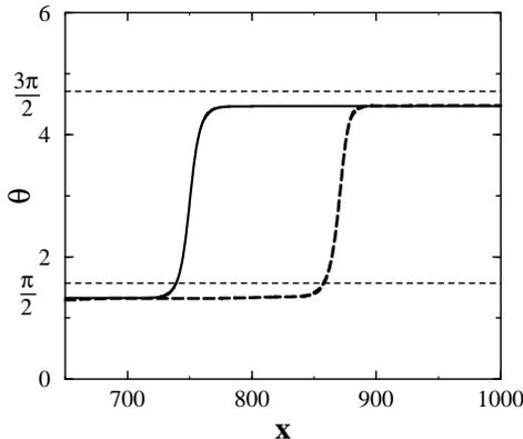
FIG. 2. The behavior of  $\pi$ -kink solution in the damped and driven SGE (14). The solid line corresponds to the initial profile  $\theta(x, 0) = V(x, 0) + \arcsin(\omega^2\eta/D)$ , with  $V$  given by (19) and  $G(\omega t)$  given by (15). The dashed line corresponds to  $t = 150$ . The parameters are  $\omega = 6$ , time step  $dt = 0.01$ , mesh size  $dx = 0.1$ , system size  $L = 1500$ ,  $\alpha = 0.03$ ,  $\eta = -0.003$ .
