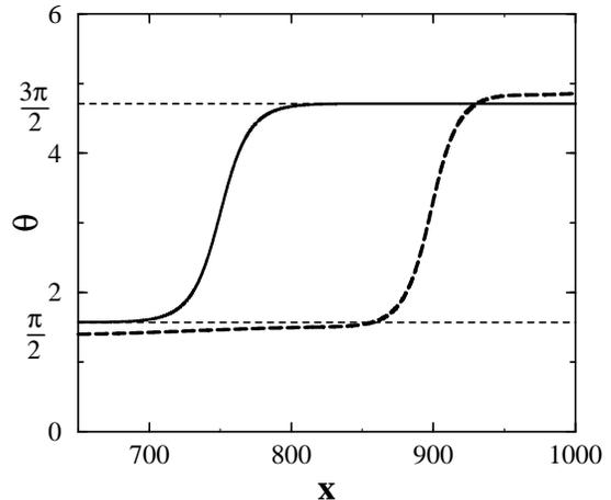
FIG. 1. The behavior of  $\pi$ -kink solution in the ac driven SGE (11). The solid line corresponds to the initial profile given by (19), with  $c = 0.5$  and  $F(\omega t) = \sin(\omega t)$ . The dashed line corresponds to  $t = 300$ . The parameters are  $\omega = 10$ , time step  $dt = 0.01$ , mesh size  $dx = 0.1$ , system size  $L = 1500$ .
