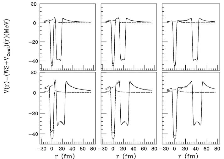
FIG. 2: Nuclear-Coulomb potentials for  ${}^8\text{B} + {}^{58}\text{Ni}$  (top) and  ${}^{17}\text{F} + {}^{208}\text{Pb}$  (bottom) at distances between the centers equal to  $d = 1.4(A_p^{1/3} + A_T^{1/3}) \text{ fm} + s$ , with  $s = 5, 15$  and  $30 \text{ fm}$ . Short and long dashed lines are the projectile and target potentials respectively. Full line is the projectile-target combined potential.
