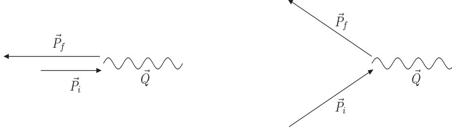
Fig. 2. The left and right parts of the figure represent kinematical configurations obtained when giving some extra momentum to the system, respectively parallel and transverse to the momentum that the initial and final states have in the Breit-frame.
