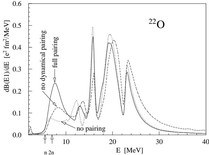
Fig. 8. Effects of the pairing correlations on the dipole response in  $^{22}\text{O}$ . The solid curve is obtained with full pairing effects included. For the dotted curve no pairing effect is included whereas in the calculation shown by the dashed curve only the static HFB potential is taken into account and the dynamical pairing effect is neglected. The TRK sum rule is satisfied for the solid and dotted curves, but not for the dashed curve.
