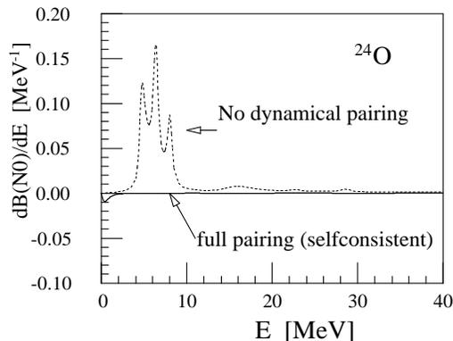
Fig. 2. The strength function for the neutron number operator in  $^{24}\text{O}$ .
