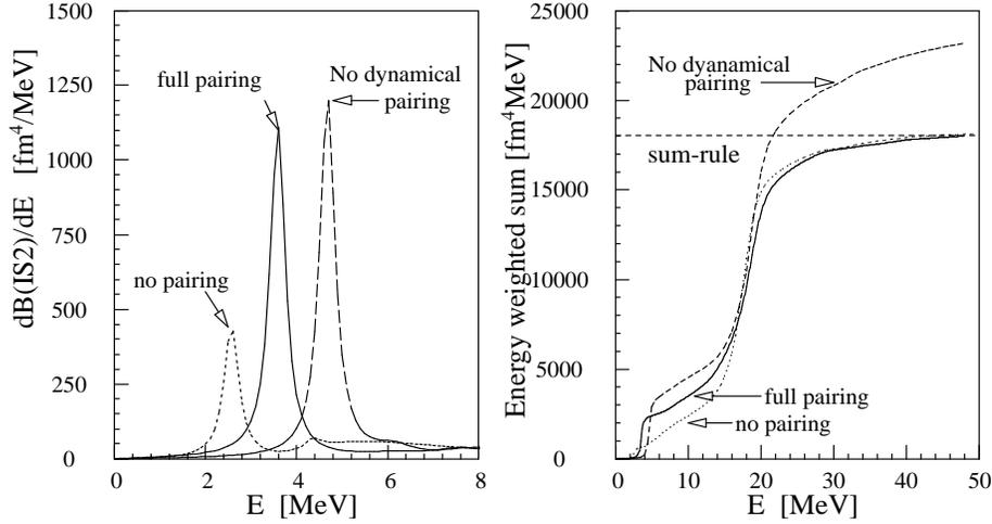
Fig. 5. Isoscalar quadrupole strength function in  $^{24}\text{O}$  (left) and its energy weighted sum (right). The calculation with the full pairing effects (solid) is compared with the one with no pairing effects (dotted), and the one where only the static HFB potential is taken into account and the dynamical pairing effect is neglected (dashed).
