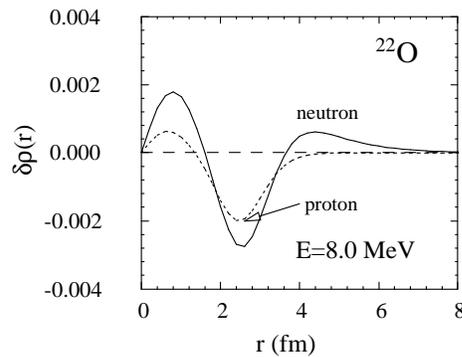
Fig. 7. The transition density for the E1 response of neutron (solid) and proton (dashed) at  $E = 8.0$  MeV in  $^{22}\text{O}$ , plotted as a function of the radial coordinate  $r$ .
