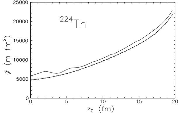
Figure 1: The deformation dependence of the rigid-body  $\mathcal{J}_{rig}$ . (curve with dots) and the cranking model  $\mathcal{J}_{cran}$  moments of inertia. The deformation parameter  $z_0$  is here the distance between the centers of left and right oscillator potentials of two-center shell model and  $m$  is the nucleon mass. The  $\mathcal{J}_{cran}$  is computed for the temperature  $T = 1 \text{ MeV}$ .
