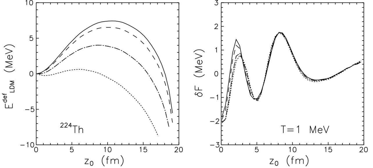
Figure 2: The liquid drop deformation energy (left) and the shell correction  $\delta\mathcal{F} = \delta R - T\delta S$  to the free energy (right) for temperature  $T = 1 \text{ MeV}$  as function of the deformation parameter  $z_0$ . The solid, dashed, dotted-dashed and dotted lines correspond to the values of angular momentum equal to 0, 20, 40 and  $60\hbar$ .
