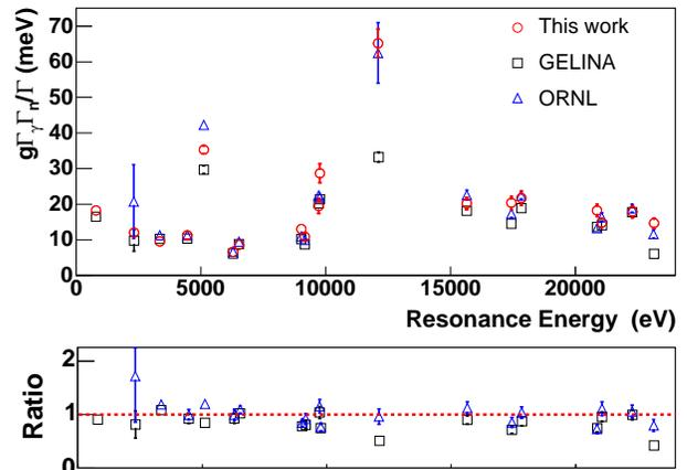
FIG. 5: (Color online) Comparison of the radiative capture kernels derived from the measurements at n\_TOF, GELINA and ORNL. The capture area shown at 2.3 keV for ORNL corresponds to an estimation reported in Ref. [6]. The capture area shown at  $\sim 12$  keV, corresponds to the sum of the three resonances in that region.
