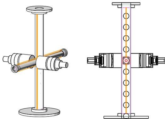
FIG. 2: (Color online) The geometry of the experimental setup used in the GEANT4 simulation of the weighting functions.
