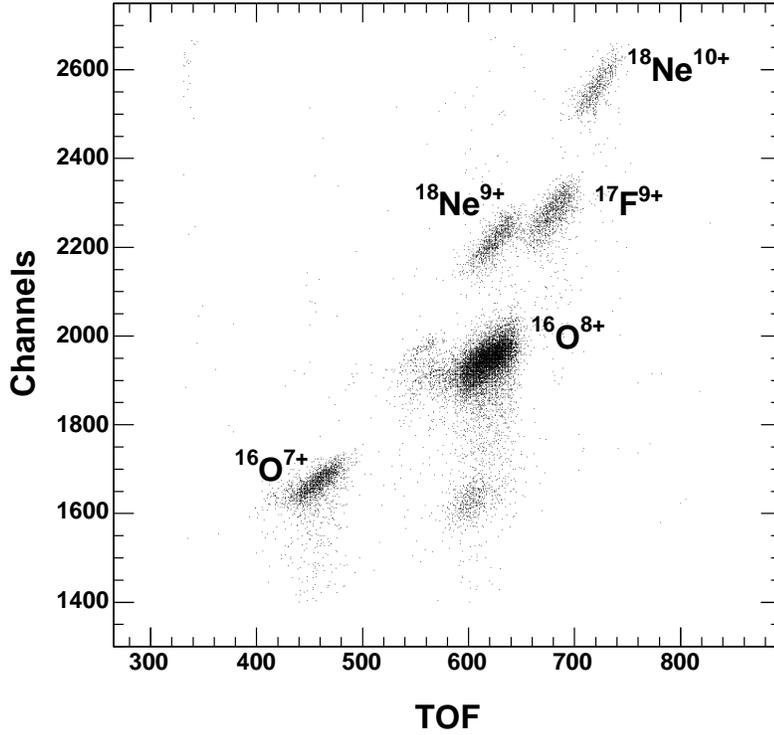
FIG. 2: Composition of the radioactive beam measured by a Si detector placed at the secondary target position. The energy of the ions is shown versus the time of flight (ToF). The “Start” signal for the ToF measurements was produced by the Si detector, and the “Stop” signal was derived from the radiofrequency (RF) signal of the buncher.
