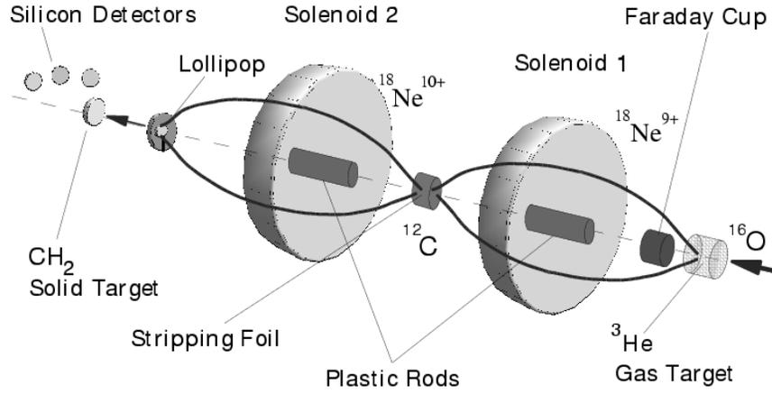
FIG. 1: The experimental setup with beam trajectories through TwinSol. The "lollipop" reduces contamination of the beam by intercepting ions that focus at a different location relative to the  $^{18}\text{Ne}$  beam.
