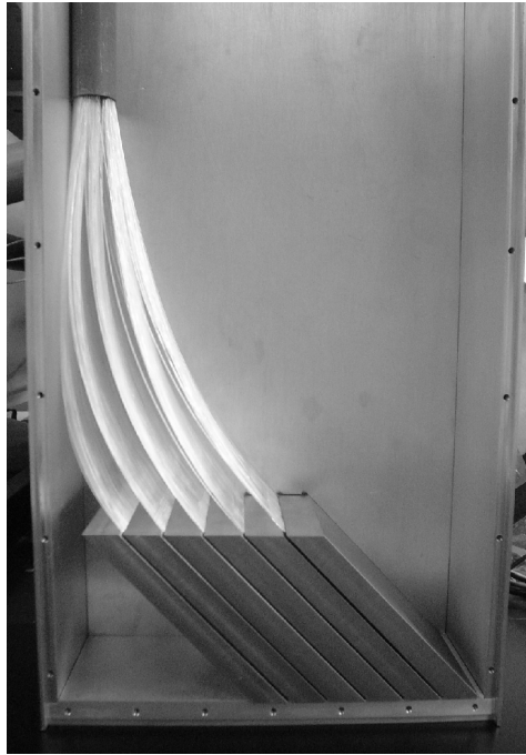
FIGURE 2. Picture showing the mechanical prototype of one longitudinal tower of the HAD section.
