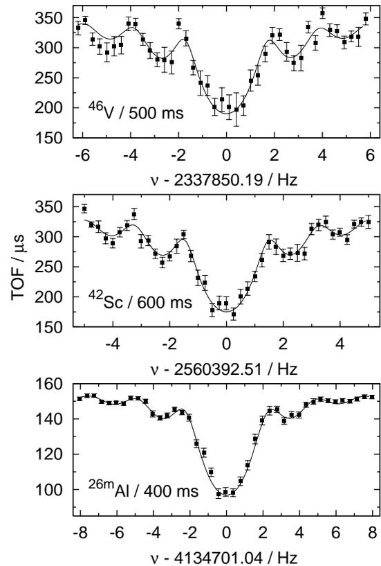
FIG. 1: Examples of the time-of-flight resonances measured for each of the superallowed beta emitters. The solid curves are fitted functions (see text).
