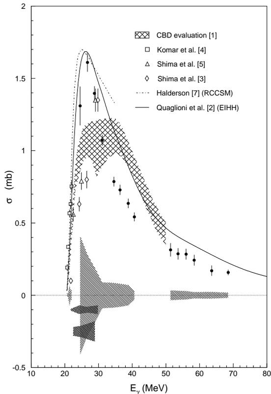
FIG. 14: The angle-integrated  ${}^4\text{He}(\gamma, n)$  cross section: present data – filled circles; CBD evaluation [1] – hatched band; RCCSM calculation [7] – dashed-dotted line; and EIHH calculation [2] – solid line. Error bars are the statistical uncertainties, while the systematic uncertainties associated with each of the data sets are represented by the bands at the base of the panel. See text for further details.
