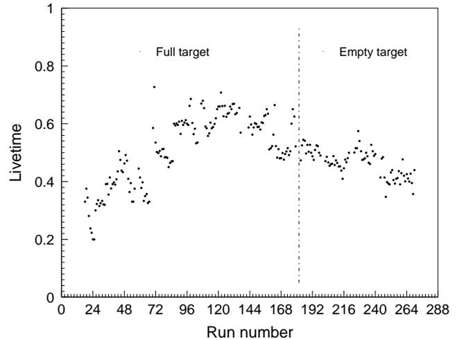
FIG. 6: The livetime efficiency correction as a function of run number. Variations in the correction are due to variations in the event rate due to different electron-beam intensities and different neutron-detector angles. See text for further details.
