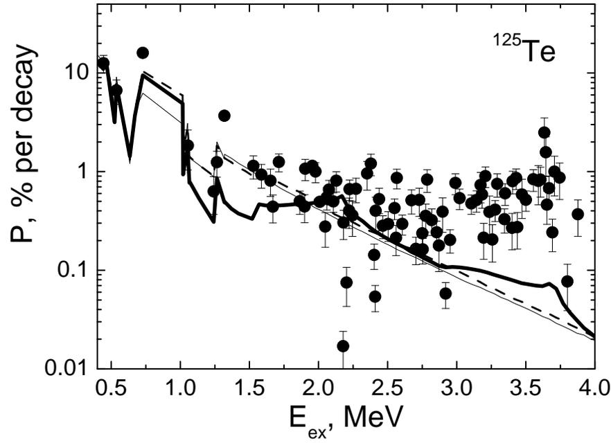
**Fig. 1.** *The total population of two-step cascades intermediate levels (points with bars), thin curve represents calculation within models [12,14]. Dashed curve shows results of calculation using data [3]. Thick curve shows results of calculation using level density [3], and corresponding strength functions of secondary transitions are multiplied by function  $h$  set by equations (1) and (2).*
