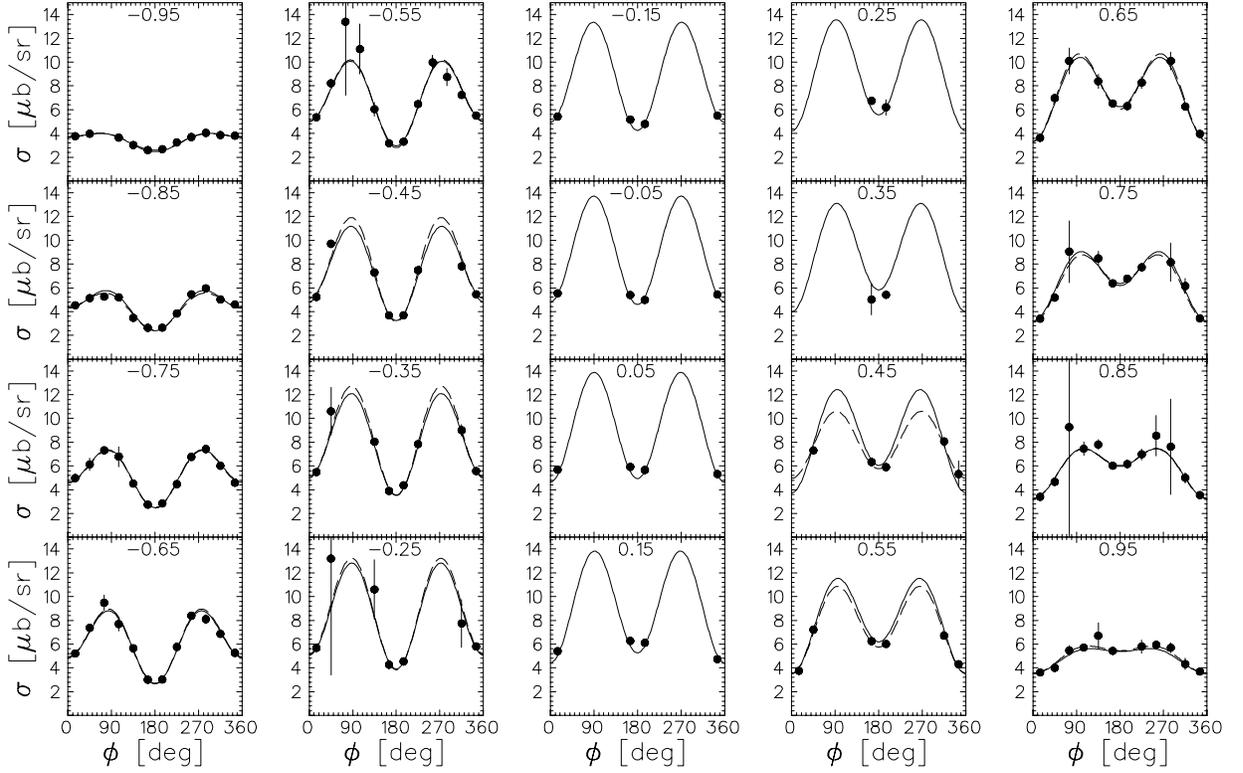
FIG. 10: Fits to the  $\phi$  dependence of unpolarized cross section data with  $(W, Q^2) = (1.23, 1.0)$ . Each panel is labeled by the central  $x$ . Solid curves fit Legendre coefficients to the entire data set shown while dashed curves fit response functions within each panel independently.
