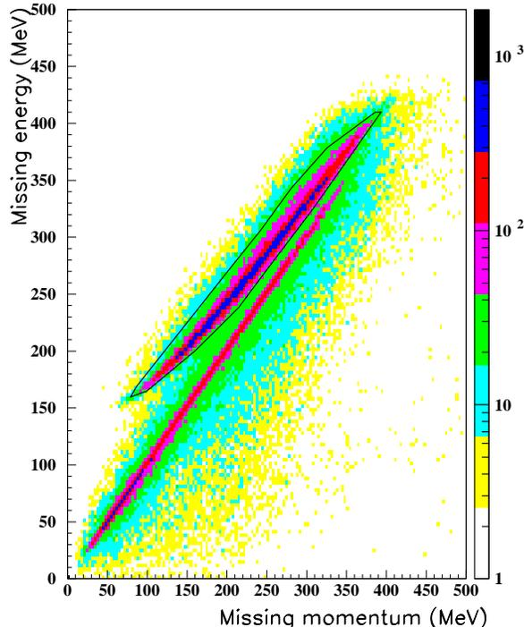
FIG. 4: (Color online) Pion production events for  $\theta_{pq} = -50^\circ$  are selected by the polygon in  $(E_m, p_m)$ . The diagonal population arises from the elastic radiative tail. The intensity scale is logarithmic.
