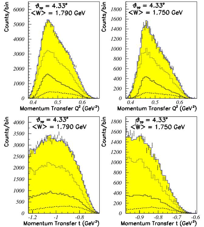
FIG. 11: Fits for two different momentum settings summed over  $\theta^*$  bins for four-momentum transfer  $t$  (top) and four-momentum transfer  $Q^2$  (bottom). Fig. 8 contains the legend explanation.
