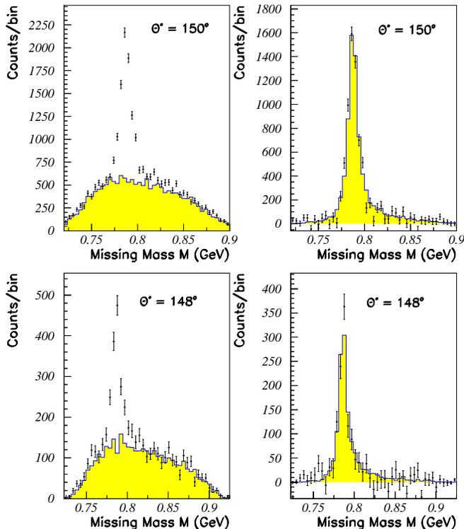
FIG. 12: The results of signal-background separation, or, equivalently,  $\omega$  yield extraction, for two different momentum settings of the hadron arm but the same,  $\theta_{\gamma p} = 4.33^\circ$ , angular setting, Top: central momentum  $p_0 = 1.077$  GeV. Bottom: central momentum  $p_0 = 0.929$  GeV.
