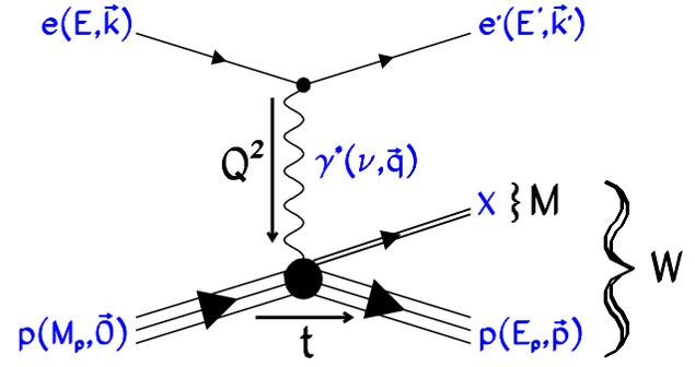
FIG. 5: Fixed target  ${}^1\text{H}(e, e'p)X$  scattering process. Here, as well as in the text below, the energy and three-momentum transfer  $\nu$  and  $\vec{q}$  are given by  $\nu = E - E'$  and  $\vec{q} = \vec{k} - \vec{k}'$ .
