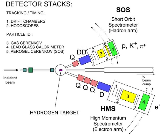
FIG. 2: Top view of Hall C. **Q** and **D** denote quadrupole and dipole magnets respectively.
