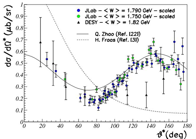
FIG. 13: The angular distributions for different average  $W$  and for  $|\phi^*| < 30^\circ$ . Error bars are statistical. The DESY data correspond to the four-momentum transfer  $Q^2 = 0.77$   $\text{GeV}^2$ ,  $W = 1.82$  GeV and full  $\phi^*$  range. The Fraas model shown here was used in the cross section extraction. Both distributions were scaled to  $W = 1.785$  GeV. The scaling procedure is described in the text.
