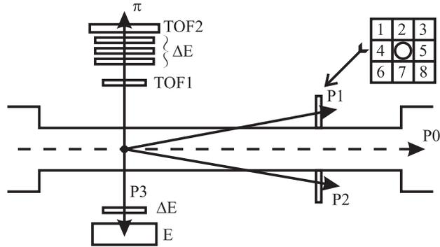
FIG. 9. The scheme of the experimental setup and its deposition on the ring of the accelerator.
