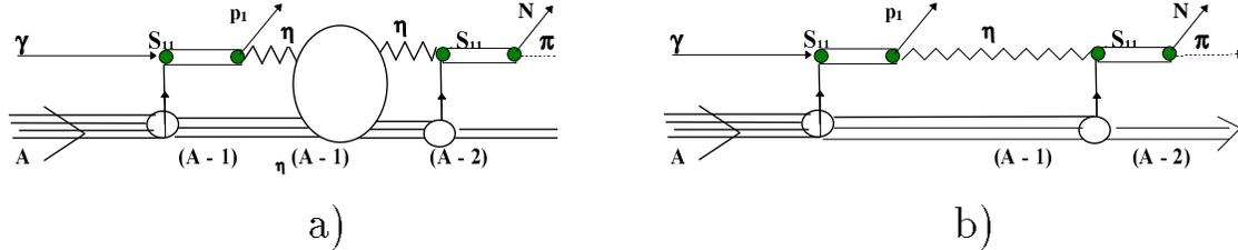
FIG. 3. (left) Mechanism of formation and decay of an  $\eta$ -nuclei in photoproduction process. ( $E_\eta \leq 70$ ) MeV. (right) Mechanism of production and annihilation of  $\eta$ 's in the nucleus. ( $E_\eta > 70$  MeV.)
