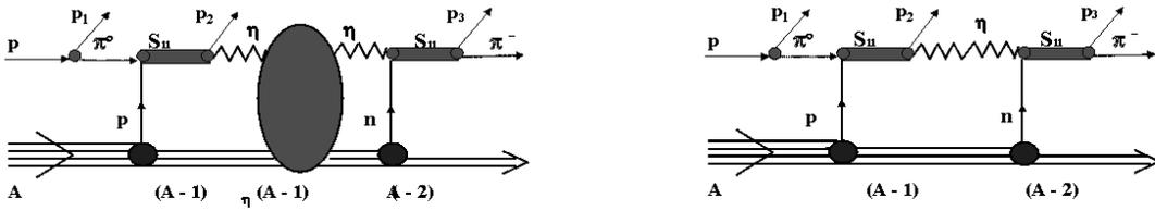
FIG. 8. (left) Mechanism of formation and decay of an  $\eta$ -nuclei in  $pA$ -collisions. ( $E_\eta \leq 70$  MeV.) (right) Mechanism of production and annihilation of  $\eta$ 's in the nucleus. ( $E_\eta > 70$  MeV.)
