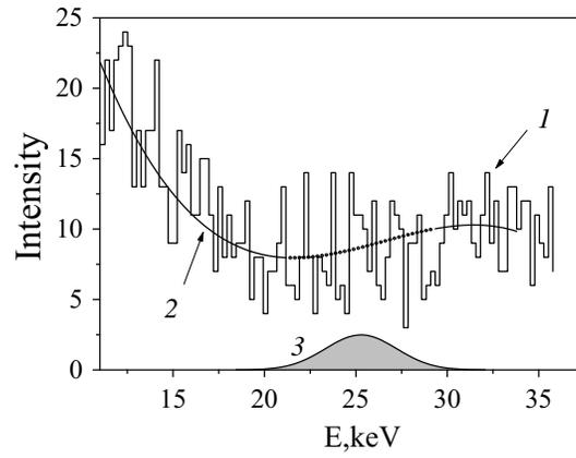
FIG. 4. (1) - Background residual energy spectrum. (2) - The best fit. (3) - Sample spectrum of an effect.
