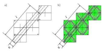
FIG. 4: (Color online) (a) Illustration of the construction of the PO channel. The black point in the upper left corner of the original billiard fixes its initial orientation. (b) The unfolding of the experimentally obtained superscarring wave function with number N=587. It has 110 wave maxima along the POC and one perpendicular to it, corresponding to the quantum numbers m=55 and n=1, respectively.
