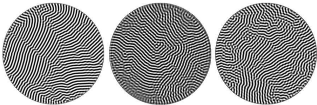
Figure 1: Images of domain chaos in Rayleigh-Bénard convection with \Gamma = 36 , \varepsilon \equiv \Delta T/\Delta T_c - 1 = 0.05 , and \Omega = 16.25 . Left: the temperature profile at the mid-plane from simulation of the Boussinesq equations with no centrifugal force. Center: shadowgraph image from experiment. A movie of this sample at 150\times actual speed is available [13]. Right: the temperature profile at the mid-plane from simulation of the Boussinesq equations including centrifugal force.
