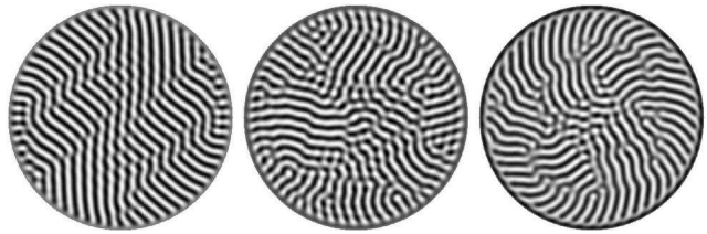
Figure 3: Simulation of the Boussinesq equations with \Gamma = 20 , \sigma = 0.93 , \Omega = 17.6 , \varepsilon = 0.055 , and an artificially large centrifugal force in order to model the effect of an inaccessible large \Gamma . Left: zero centrifugal force. Center: centrifugal force is 4 times the physical value. Right: centrifugal force is 10 times the physical value. A movie of this sample at 100 \times actual speed is available [28].
