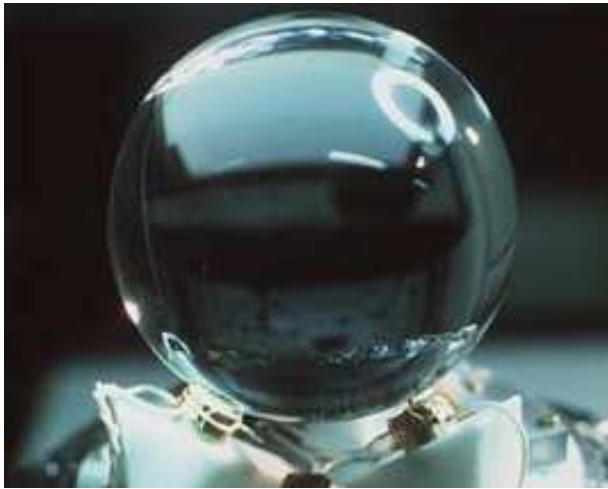
FIG. 7: Quartz sphere with supporting transducers.
