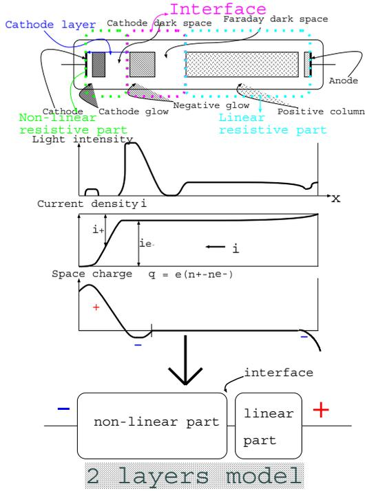
Figure 1: Schematic figure of 2 layers model for glow discharge. We consider that the glow discharge structure consists of two parts, the non-linear resistive region and the linear one.
