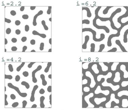
Figure 19: Stripe patten. Spots are extended and connected to form a *string*. As  $i_u \nearrow$ , many strings are formed, and as a result they are connected with the neighboring strings as shown. Plotted for  $i_u = 6.2, 8.2$  (*stripe*).
