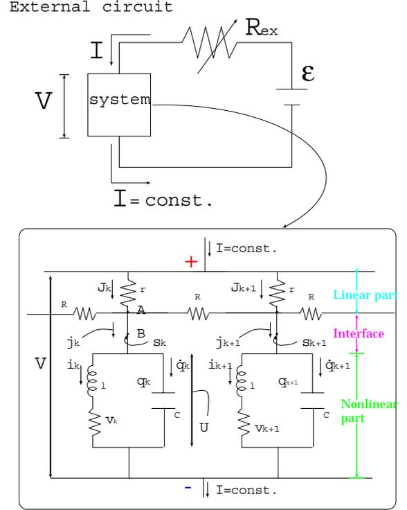
Figure 2: Schematic figure of our 2-dimensional discharge model. Our model system consists of  $N$  coupled circuits. The element  $k$  is connected with neighbor ones by linear resistor  $R$  and with “External circuit”. Although displayed in a one-dimensional representation, what we actually simulated in the paper is a two-dimensional case.
