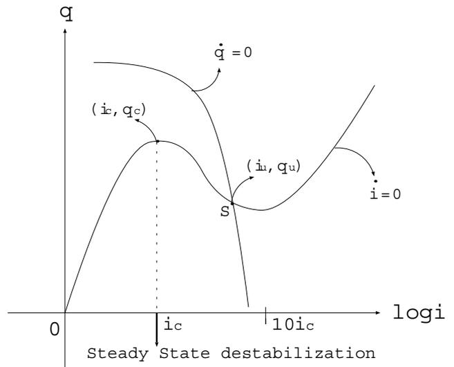
Figure 3: Nullcline of the single element dynamics. Parameter  $a (= r \frac{i_c}{v_c})$  is chosen so that the steady state  $(i_u, q_u)$  is destabilized when  $i_u > i_c$ , and the element shows limit cycle oscillation.
