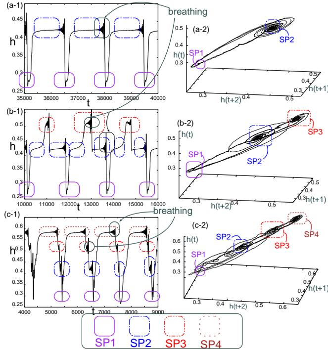
Figure 11: (a) The case  $M_2$  ( $i_u=0.93$ ), (b) The case  $M_3$  ( $i_u=0.939$ ), (c) The case  $M_4$  ( $i_u=0.98$ ), (1) Time series of  $h$ , (2) The embedded orbit of  $h$  into 3 dimensional phase space.  $h$  has a sole value corresponding to each state  $sp_1 \sim sp_4$  with respect to different  $i_u$  under fixed  $D$ .  $D = 0.014$
