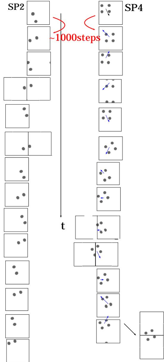
Figure 10: A sequence of snapshots for  $sp_2, sp_4$  state. We see that the positions of  $sp_2, sp_4$  shift in time due to the asymmetry for splitting. In a long time scale, the clusters appear to be wandering.  $sp_2:i_u = 0.93$ ,  $sp_4:i_u = 0.98$ ,  $D = 0.014$
