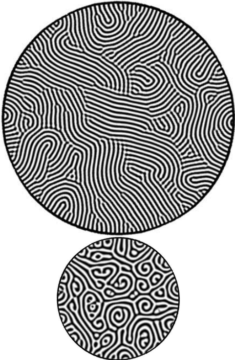
FIG. 2: Numerical simulations of two large-aspect-ratio cylindrical convection layers. The pattern is illustrated by contours of the thermal perturbation, dark regions represent cool descending fluid and light regions warm ascending fluid. Both simulations are initiated from random thermal perturbations and the lateral sidewalls are insulating. (Top) \Gamma = 57 , \sigma = 2.94 , R = 2169.2 and t = 74\tau_v . (Bottom) A spiral defect chaos state, \Gamma = 30 , \sigma = 1.0 , R = 2950 and t = 254\tau_v .
