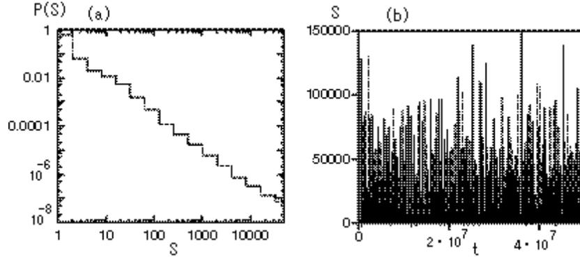
Figure 7: (a) Histogram of size distribution of the total displacement  $S = \sum_{i=1}^N \Delta x_i$  during each slip event at  $\beta = 1$  in logarithmic scales. (b) The total displacement  $S$  as a function of the event time at  $\beta = 1$
