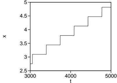
Figure 1: Time evolution of  $x$  in a single block and spring system eq. (1) at  $M = 1$ ,  $\alpha = 1$ ,  $\beta = 1$ ,  $\sigma = 1$ ,  $K = 10$ ,  $V = 0.001$  and  $F_s = 3$ .
