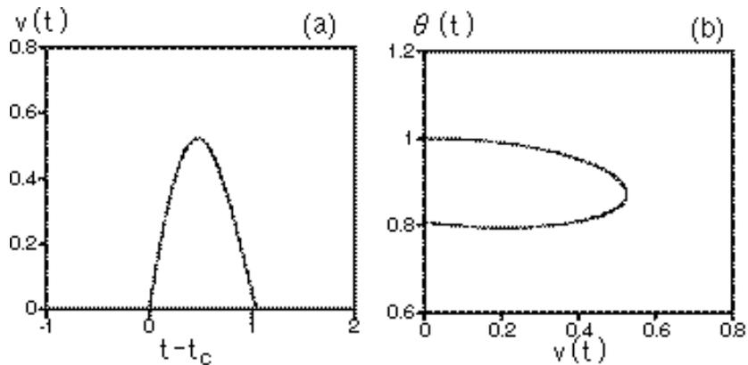
Figure 2: (a) Time evolution of  $v = dx/dt$  in a slip process for a single block and spring system at  $M = 1$ ,  $\alpha = 1$ ,  $\beta = 1$ ,  $\sigma = 1$ ,  $K = 10$ ,  $V = 0.001$  and  $F_s = 3$  (solid curve) and the time evolution by eq. (3) (dashed curve). The two curves are overlapped and the difference is invisible in this plot. (b) Phase portraits of  $(v(t), \theta(t))$  by eq. (1) (solid curve) and by eq. (3) (dashed curve). Two curves are also well overlapped.
