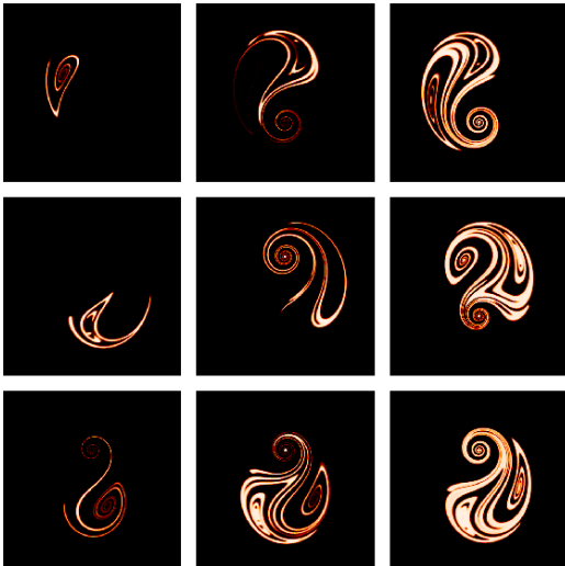
FIG. 5. Time evolution of the activator concentration under the open flow. The snapshots are shown every 0.7 time units, from top to bottom and then from left to right, starting 0.7 time units after the initial perturbation, Da = 50 and Pe \approx 56 . After the last time shown, excitation is maintained indefinitely in the system, and the long-time pattern, which follows the shape of the unstable manifold of the chaotic saddle, repeats periodically in synchrony with the flow.
