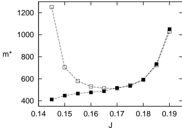
FIG. 5. Dependence of the effective mass of the mobile breathers with the coupling parameter for  $\theta_{tw} = 180^\circ$ . The blank squares correspond to mobile breathers obtained from static one-site breathers. Full squares are obtained from static two-site breathers.
