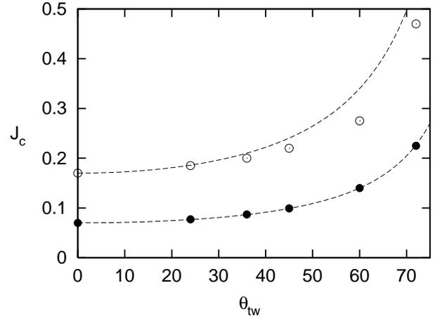
FIG. 4. Range of stability of the one-site (circles) and two-site (full circles) breathers as a function of the twisting angle in degrees.  $J_c$  is the maximum value of the coupling parameter for which the breather is stable. The dash lines represent the values calculate within the NNI approximation.  $J_c$  is in dimensionless units.
