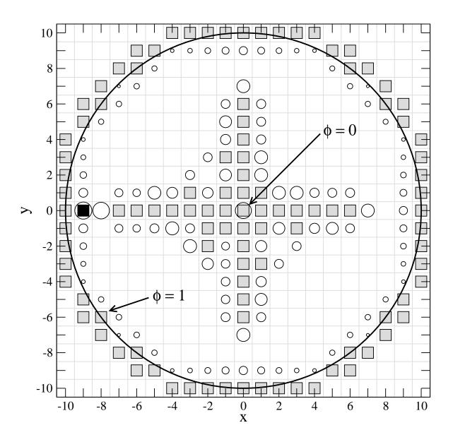
Figure 2: Discharge channel, for a 20 x 20 square lattice, showing the attachment between the return branch (outer gray boxes) and the main branch (inner gray boxes).
