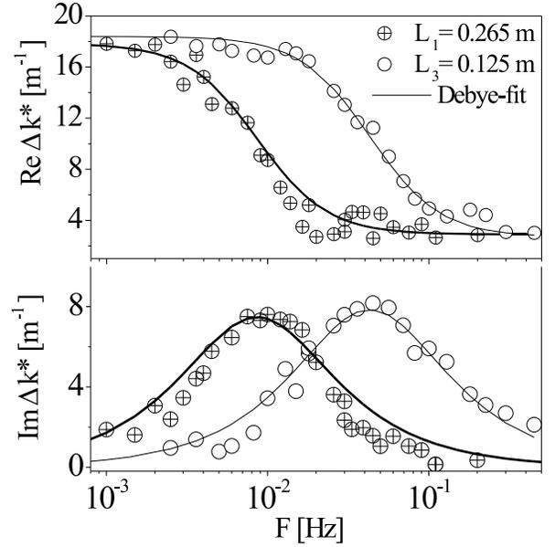
FIG. 4. Frequency "dispersion" of the real and imaginary parts of  $\Delta k^*$  as obtained from modulation experiments of type (ii) for the two different container diameters  $L_1 = 265$  mm and  $L_3 = 125$  mm ( $f = 90$  Hz,  $k_0 = 1480$   $\text{m}^{-1}$ ,  $\varepsilon = 9\%$ ). Solid curves are fits according to the Debye relaxator
