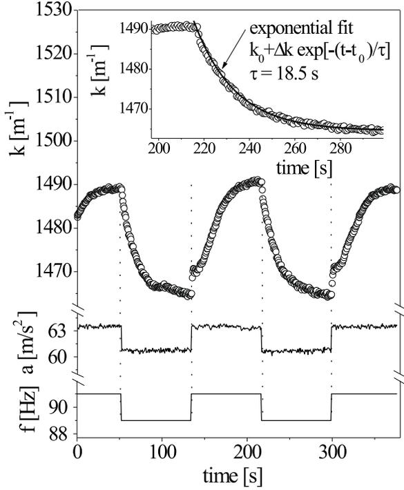
FIG. 2. Temporal decay of the wave number  $k(t)$  in response to a step-like [type (i)] change of the drive frequency  $f$ . Also the drive amplitude  $a$  was changed to keep the reduced amplitude  $\varepsilon = a(t)/a_c[\omega(t)] - 1$  constant. The decay of the wave number  $k(t)$  could be fitted by an exponential. (Parameters:  $L = 0.265$  m,  $\varepsilon = 9\%$ ,  $f = 90$  Hz)
