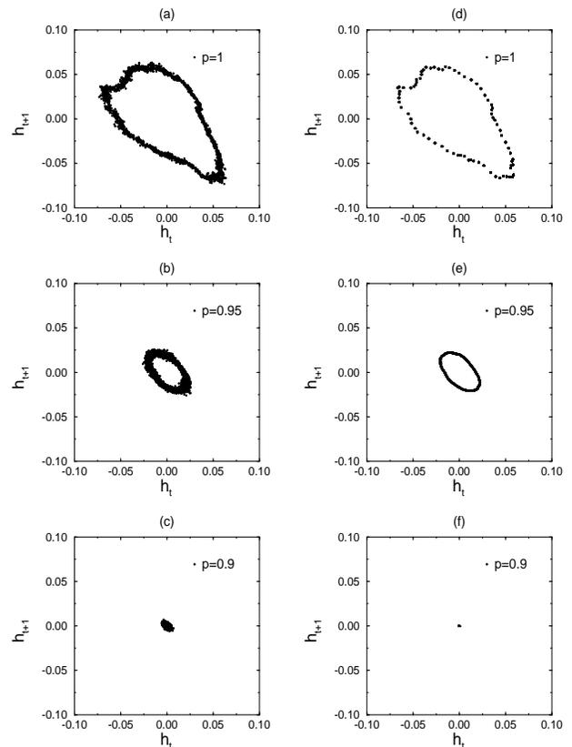
FIG. 2: Examples of the return maps of the mean field are shown ( $a = 1.625$ ,  $K = 0.4$ ). While (a), (b), and (c) are obtained by the direct numerical calculation of (8) with the size of  $N = 10^5$ , (d), (e), and (f) are obtained by the numerical calculation of (11) with  $2^{18}$  grids. (a) and (d) are for  $p = 1$ , (b) and (e) are for  $p = 0.95$ , (c) and (f) are for  $p = 0.9$ . We plot 2000 points after  $10^4$  steps as transient.
