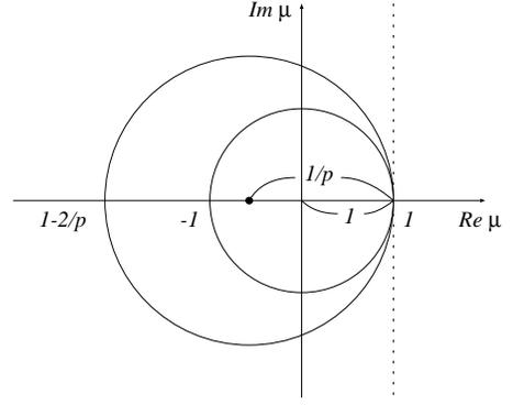
FIG. 4: The stability condition. If all solutions  $\mu_i$  of (26) lie within the large (unit) circle, the stationary state is stable for  $p < 1$  ( $p = 1$ ). Thus, all  $\mu_i$  lie on the left of the dotted line, there exists threshold value  $p_c$ .
