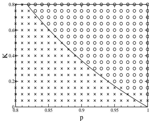
FIG. 5: Phase diagram of the collective motion for  $a = (1 + \sqrt{5})/2$ . The numerical results are obtained by calculation of (11) with  $2^{18}$  grids. Circles and crosses represent the cases of  $\langle h^2 \rangle^{1/2} > 10^{-12}$  and  $\langle h^2 \rangle^{1/2} < 10^{-12}$ , respectively. The solid line represents the theoretical prediction (33).
