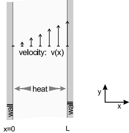
FIG. 1. Graphical illustration of the shear flow. The system is confined between two walls at positions  $x = 0$  and  $L$ . The walls move relative to each other in the  $y$  direction, thus inducing a velocity profile  $v(x)$  indicated by vertical arrows. For a fixed temperature at the walls this leads to an accompanying heat flow in the  $x$  direction (gray arrows).
