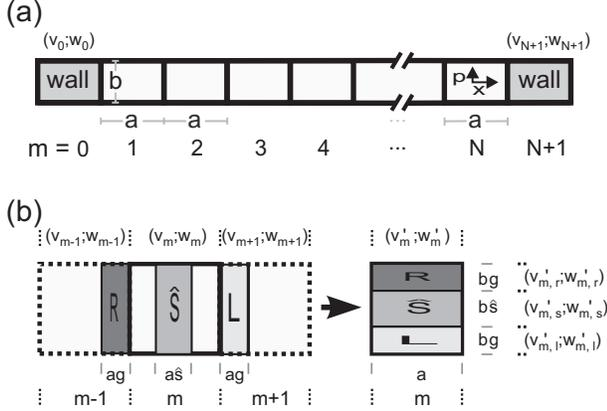
FIG. 3. Graphical illustration of the  $(x, p)$  multibaker representation of the laminar flow. (a) Domain of the map. The outermost cells (indicated as grey boxes) are again used to implement boundary conditions. (b) Action in the bulk. The average values of the fields  $v(x, y)$  and  $w(x, y)$  on the cells [cf. Eqs. (12) and (18)] and strips [cf. Eqs. (11) and (19)] are given on the margins.
