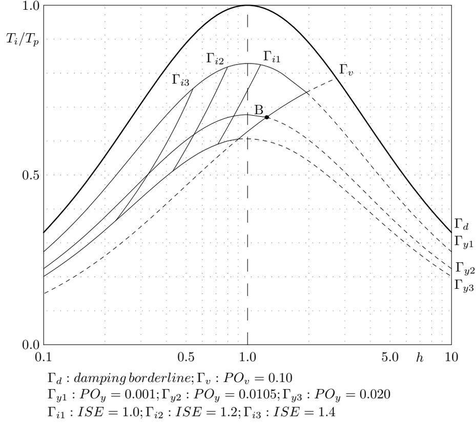
FIGURE 2. Tuning chart of systems without time delay
